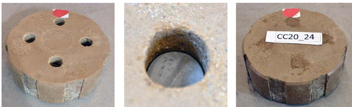
Figure 5-5. Final preparation of a bentonite block. Left image shows how the block has been given its final shape with grooves made to fit with the titanium cage and holes drilled for the small specimen cylinders. In the centre image a cement cylinder has been placed in the small hole and the right image finally shows how the holes have all been filled with bentonite powder of the same type as the bentonite block itself.
