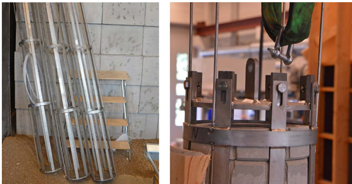
Figure 4-1. The lower part of three of the titanium cages used in the field scale bentonite experiments (left image) and the top part with the adjustable section and lifting eye (right image).
