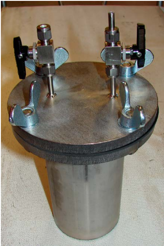
Figure 4-4. The stainless steel container used in the laboratory scale experiments.
