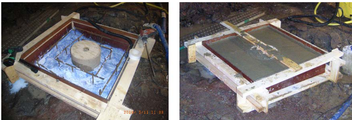
Figure 3-4. Casting of the base for one of the experiments in NASA0507A.
