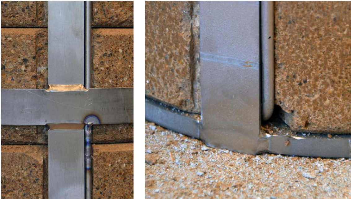
Figure 4-3. Images showing details of the titanium tubes used to distribute the water in the sand surrounding the bentonite blocks. The left image shows how the tubes are attached by means of welding to the titanium cage and the right image shows the bottom plate with the titanium tube placed in a slit in the lowermost bentonite block.
