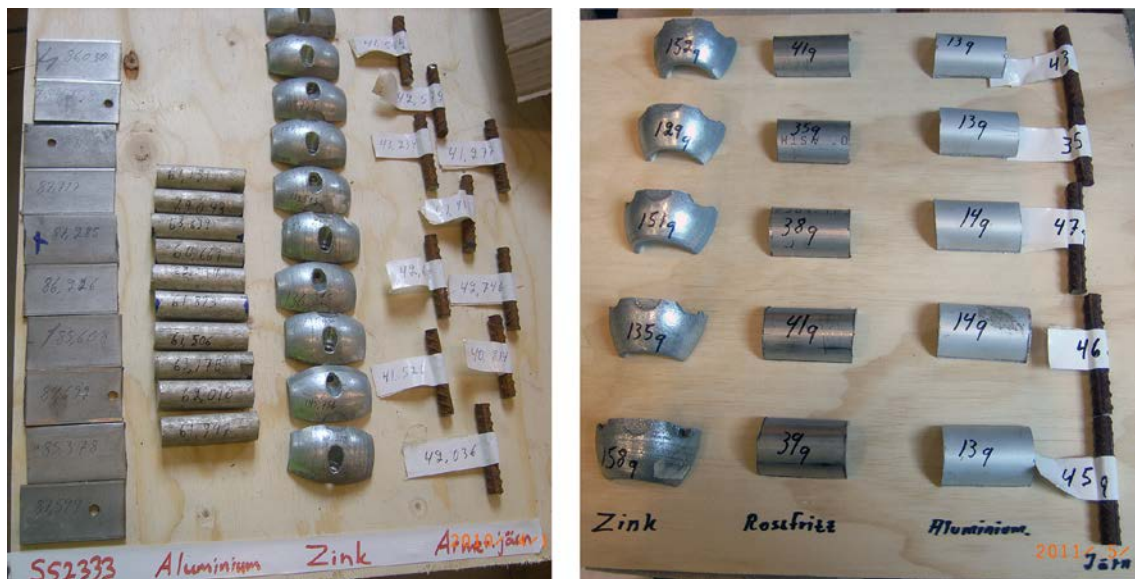
Figure 5-1. Metallic specimens used in the field scale concrete experiments deposited in NASA0507A (left image) and NASA2821A (right image).
