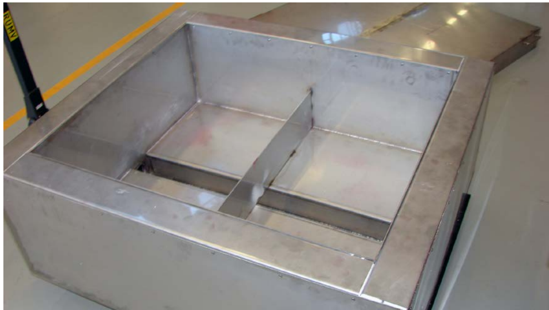
Figure 4-5. The heated water bath used to heat some of the containers in the laboratory scale experiments to about 50°C.
