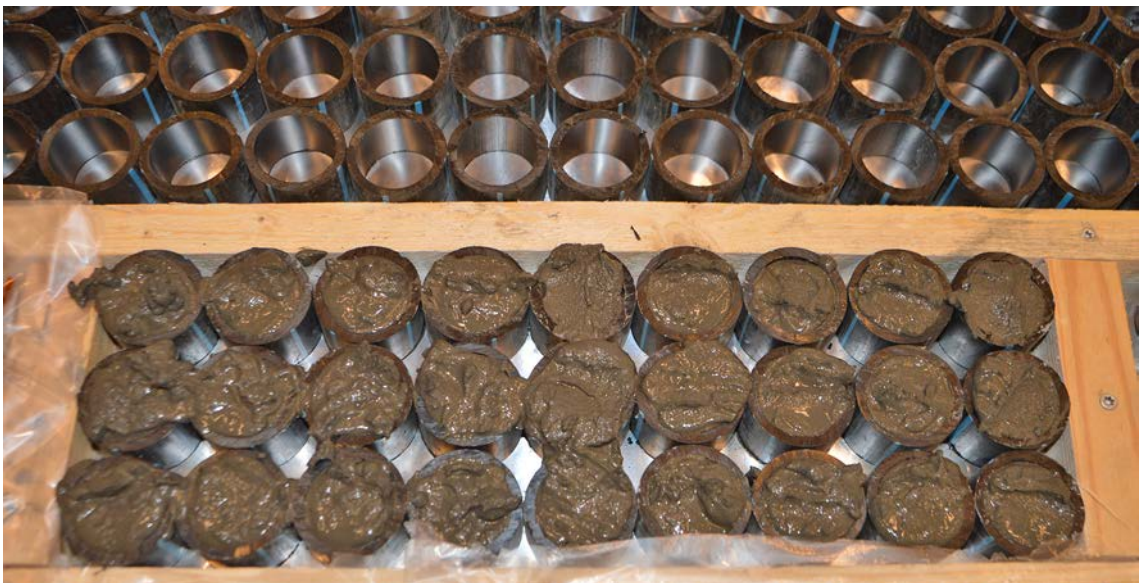
Figure 5-4. Casting of the paste specimens.
