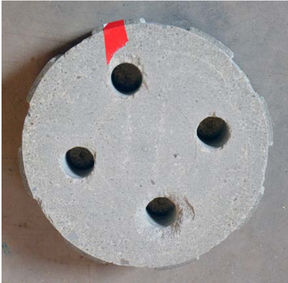
Figure 5-3. The final shape of a bentonite block with holes for the material specimens and grooves made to make the block fit into the titanium cage. The red tape which corresponds to North in the bentonite package was removed when the package was assembled.
