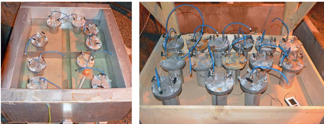
Figure 6-12. The steel containers in the heated bath (left image) and placed under a protective cover in NASA2861A (right image). During operation a lid is placed on the heated bath for insulation.
