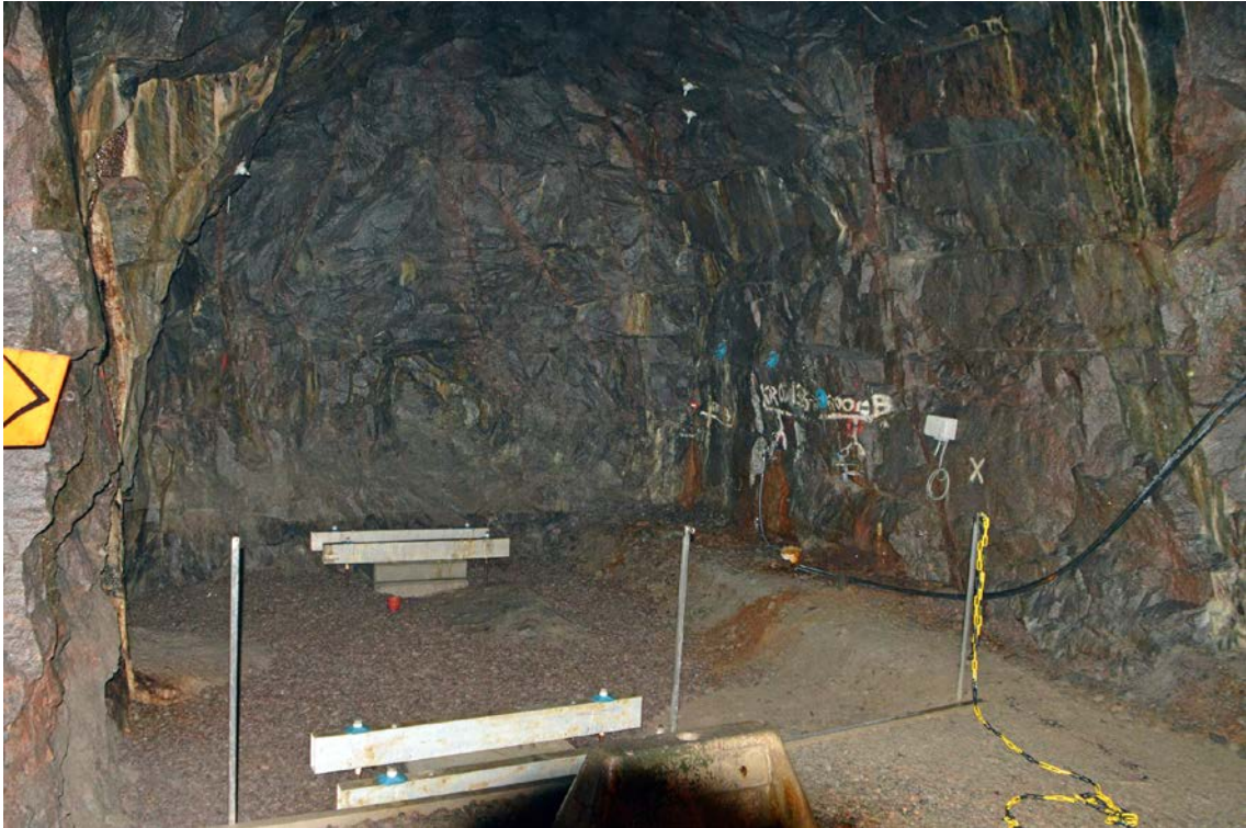
Figure 6-4. Both experiments in NASA0507A are ready and the lids bolted to the bedrock.
