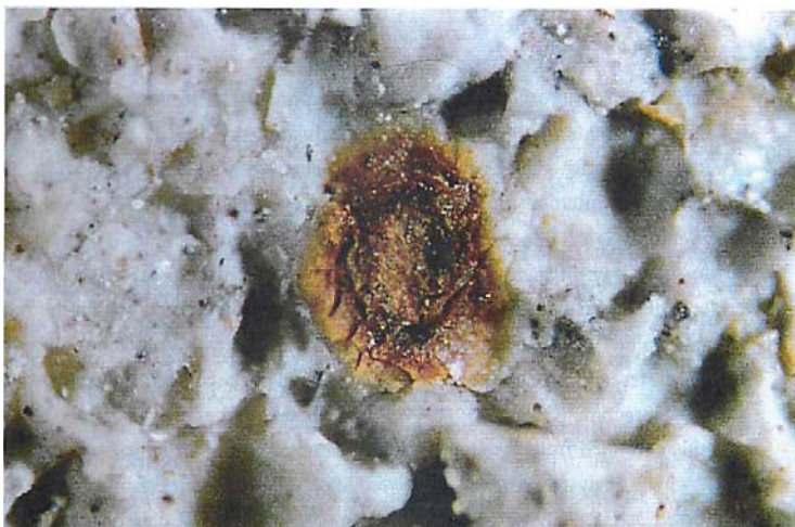
Figure 3-4. Oxidised pyrite particle in MX-80 bentonite (after Melamed and Pitkänen 1994). The diameter of the oxidised particle is approximately 800 \mu\text{m} .
