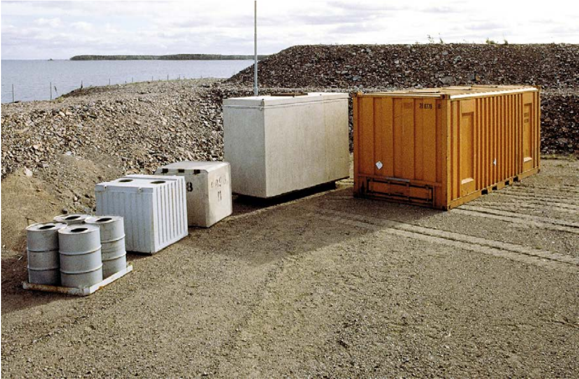
Figure 1-2. The different waste containers used to encapsulate the waste in SFR 1.
