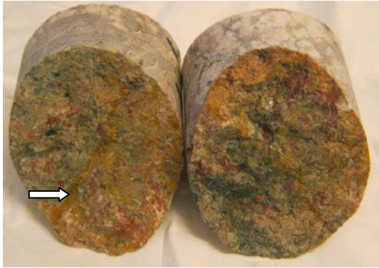
Photo of fracture surface with rust-brown colour.
