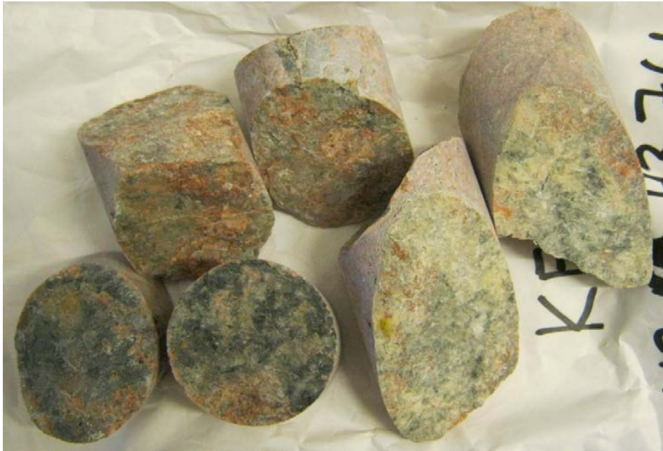
Figure A1-35. Photo of the sampled fractures from KFR104 43.53–43.76 m.
