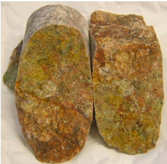
Figure A1-63. Photo of the sampled fracture from KFR104 328.75–328.86 m.
