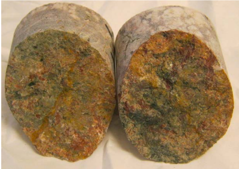
Figure A1-18. Photo of the sampled fracture from KFR104 25.03–25.09 m.
