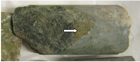
Photo of fracture surface with rust-brown mineral coating.
