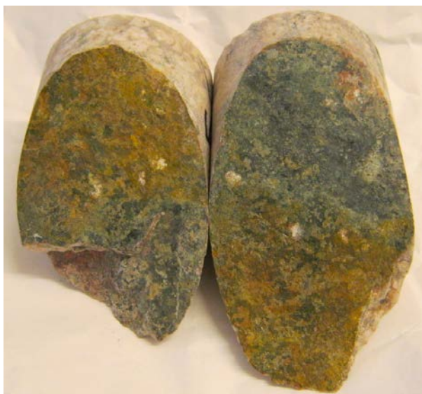
Figure A1-21. Photo of the sampled fracture from 25.51–25.62 m.
