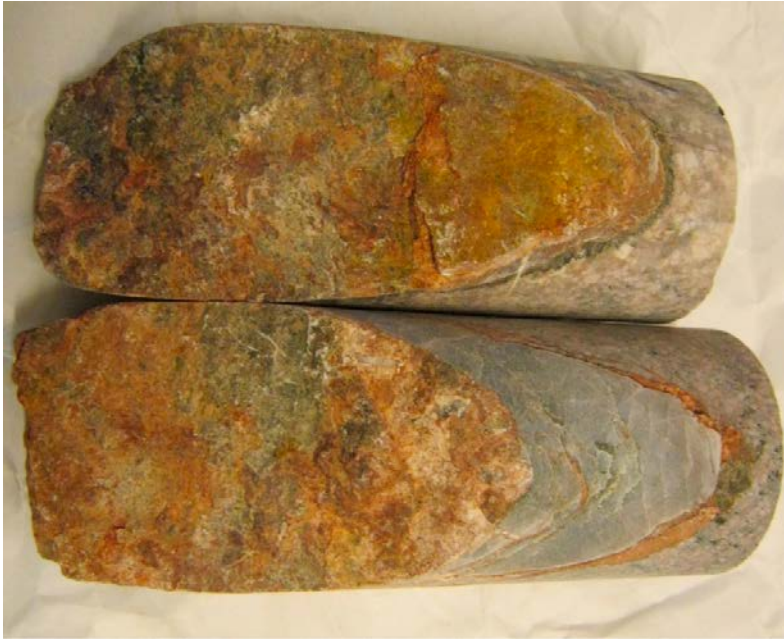
Figure A1-50. Photo of the sampled fracture from KFR104 107.64–107.83 m.
