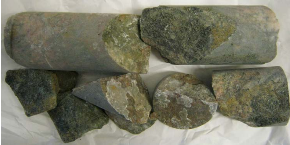
Figure A1-6. Photo of the sampled fractures from KFR102B 113.56–113.88 m.
