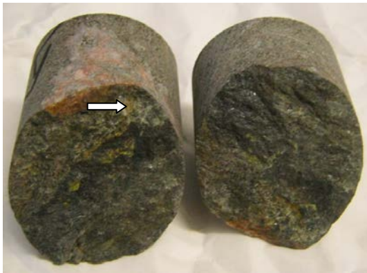
Photo of fracture surface green-yellow mineral coating.
