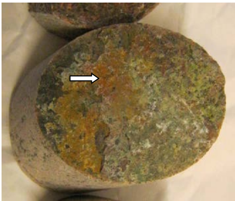
Photo of fracture surface with rust-brown mineral coating.
