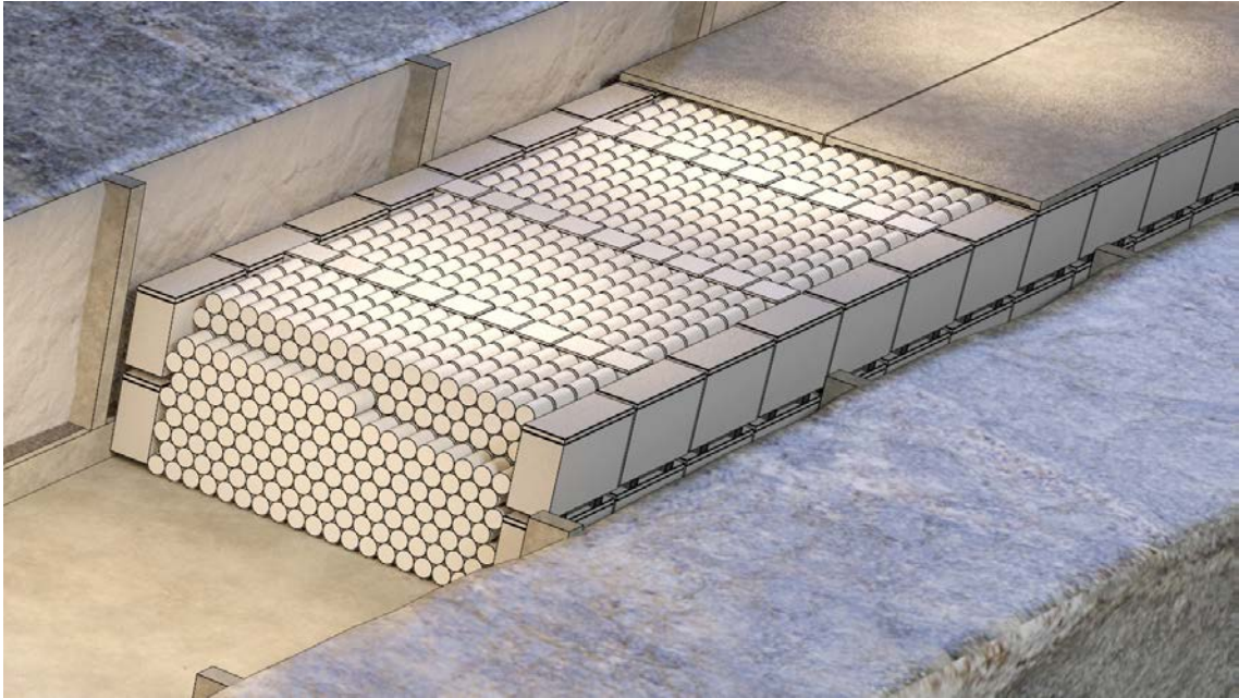
Figure 3-7. Detail of sections with drums in 1BTF.
