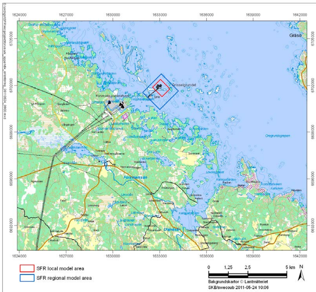
Figure 1-1. Location of Forsmark in norther Uppland. The lower map shows the boundaries of the SFR local and regional model area, respectively, and the location of the SFR 1 facility. The local model area (or domain) covers the volume that hosts SFR 1 and SFR 3, whereas the regional model domain places the description of the local domain in a larger context (SKB 2013).
