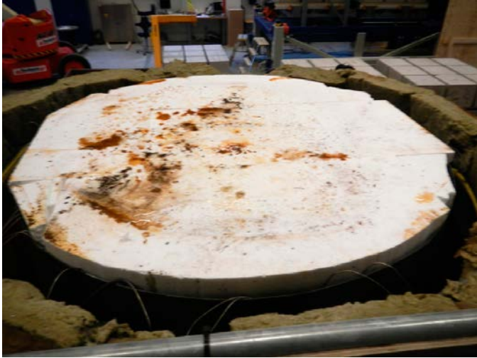
Figure 4-7. Some puddles of water between the upper layer of insulation and the steel lid.
