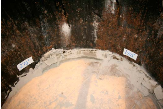
Figure 4-14. The “wet” bentonite at the bottom of the test cylinder.
