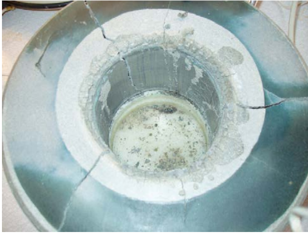
Figure A1-6. Radial cracking seen on specimen SB1 at termination.
