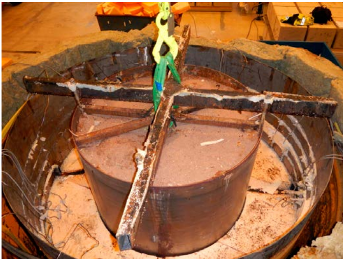
Figure 4-8. The heater lifted up from the test cylinder.
