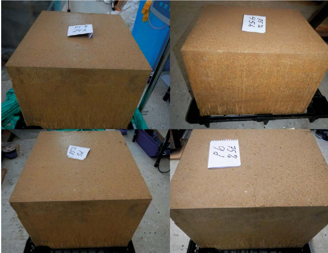
Figure 6-27. Photos of the block placed in 75% taken at different times (24 h, 45 h, 5 days and 9 days) after test start. (There is a small damage on the bottom-left side of the block due to the block handling before test).
