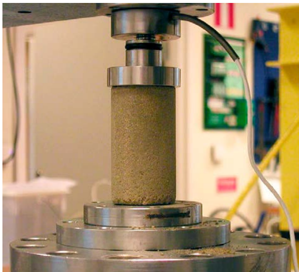
Figure 6-8. Test arrangement for determination of the shear strength of pre-compacted samples of backfill material.
