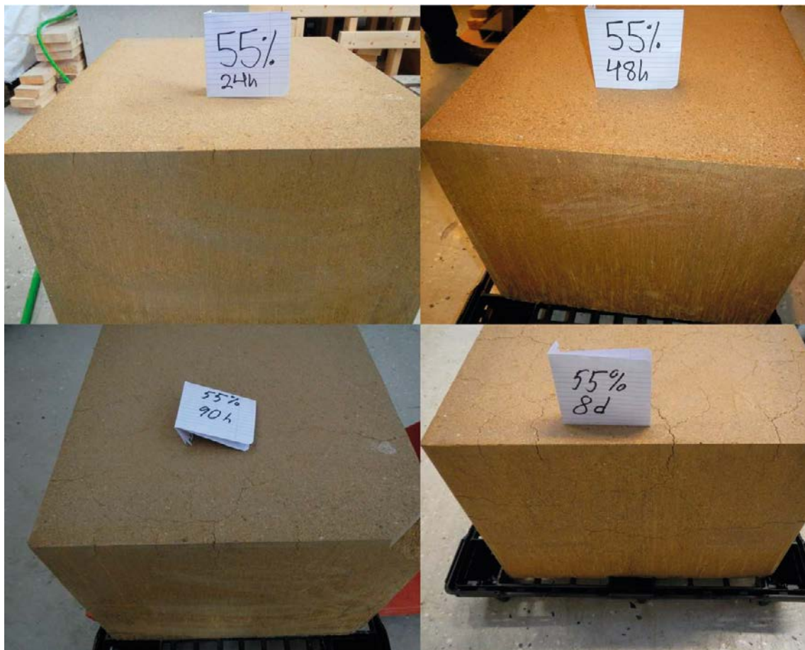
Figure 6-26. Photos of the block placed in 55% taken at different times (24 h, 48 h, 90 h and 8 days) after test start.
