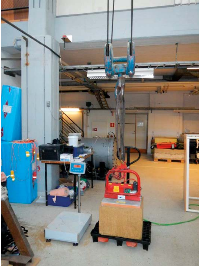
Figure 6-23. Photo showing a block taken out from a climate chamber for control. A vacuum lifting device is used to lift the block from the pallet to the balance.
