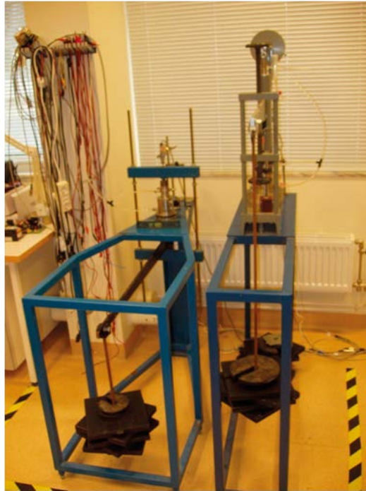
Figure 6-4. Left: Schematic drawing of the test cell. Right: Photo of the test equipment used for the oedometer tests.
