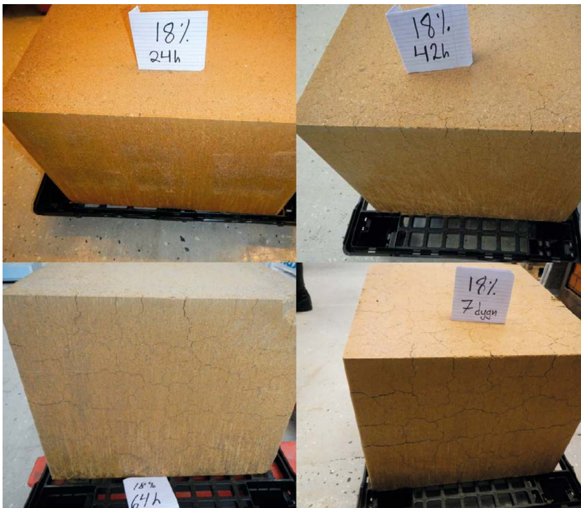
Figure 6-25. Photos of the block placed in 18% RH taken at different times (24 h, 42 h, 64 h and 7 days) after test start.
