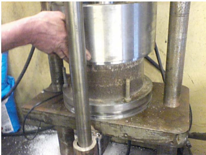
Figure 2-8a. Compaction of blocks. G001-L bentonite block with 285 mm diameter and 120 mm height. The black colour is molybdene disulphide for lubricating the form. Density 2,035 kg/m 3 .
