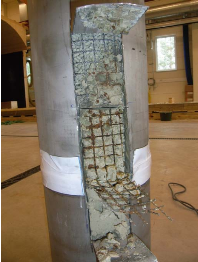
Figure 2-5. The tube and cage cut open for sampling. The clay grains are seen in the upper part while they are embedded in mud in the lower part.
