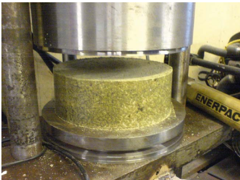
Figure 2-8b. Compaction of blocks. CEBOGEL bentonite block with 285 mm diameter and 100 mm height. Density 2,060 kg/m 3 .
