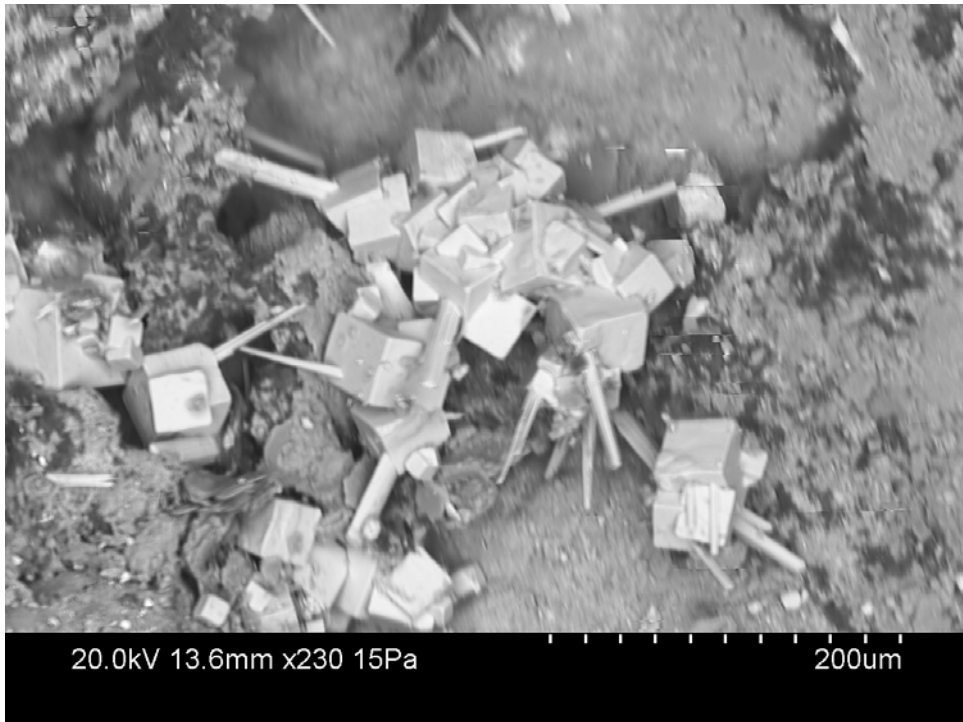
Figure A5-5. Backscattered electron image of cubic- and needle-shaped pyrite crystals on mixed layer clay.
