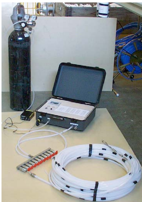
Figure 4-3. Air-lift pump equipment used in small diameter standpipes.
