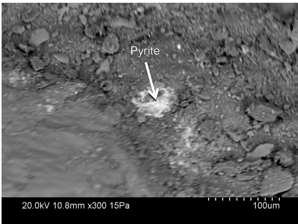
Figure A5-44. Backscattered electron image of pyrite on albite and mixed layer clay (Fracture 1).
