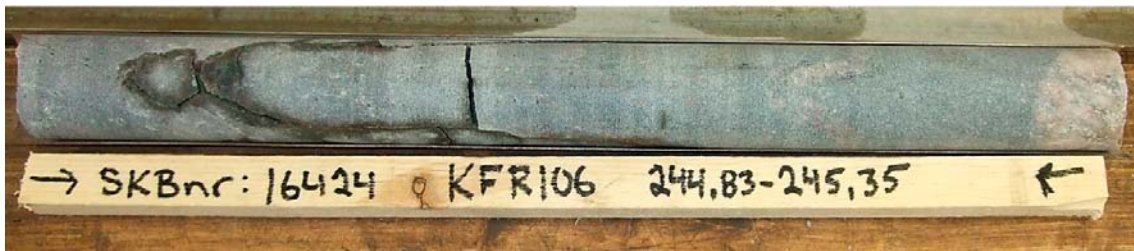
Figure A5-39. Photograph of drillcore sample.
