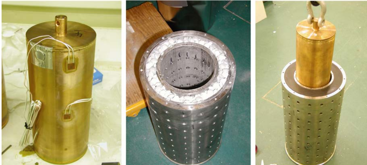
Figure 2-3. Left: Strain gauges mounted on model canister; Centre: Positioning of bentonite pellets inside annulus of support cage; Right: insertion of model canister assembly into support cage.
