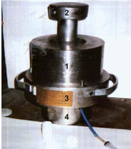
Figure A4-2. Pore fluid expression device. CSIC equipment (Hidalgo et al. 2005b).
