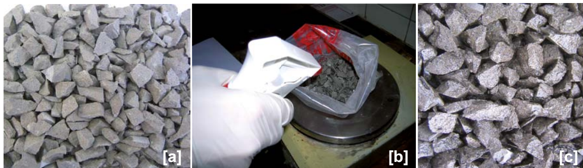
Figure 3-3. Sample pre-conditioning procedure (CO 2 -free deionised water addition). (a) Initial surface of dry sample, (b) water spraying, (c) surface of wet sample.
