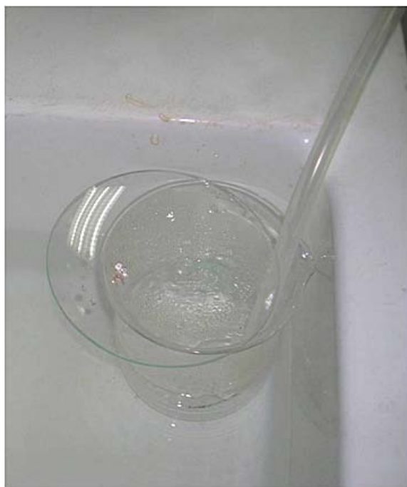
Figure 3-2. Cooling procedure for CO 2 -free deionised water. The glass beaker is partially covered by a watch glass and N 2 (optionally Argon) gas is bubbled through the solution using a plastic tube.
