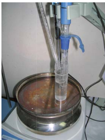
Figure 2-3. Pore fluid pH measured with a pH electrode under inert atmosphere.
