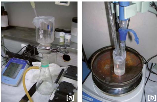
Figure 2-8. Filtering and pH measurement procedure in the routine (ESL) method with filtering. (a) N_2 (optionally Argon) gas is passed through the head space of the filtering apparatus. A peristaltic pump is used to assist filtration with the pore water sample collected in the bottom flask. (b) N_2 (optionally Argon) gas is passed through the head space of the vessel with a temperature sensor and combination pH electrode in the stirred pore fluid sample.
