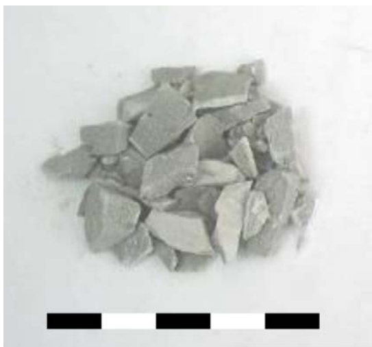
Figure 2-1. Particle size required in the reference (PFE) method. The black-and-white scale is five mm.
