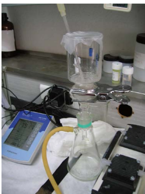
Figure 3-7. Stirring and filtration procedures followed in the routine (ESL) method with filtering. Filtering the suspension is conducted under N_2 (optionally Argon) gas.
