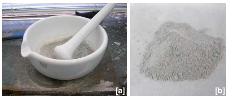
Figure 2-5. Powdered particle size required in both routine (ESL) methods. (a) The sample is ground with a pestle and mortar to obtain (b) a particle size diameter, \phi \approx 80 \mu\text{m} .
