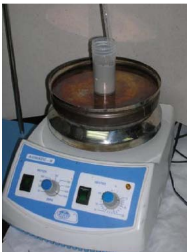
Figure 2-6. Initial stirring procedure used in both routine (ESL) methods. The suspension is stirred while N 2 (optionally Argon) gas is passed through the head space of the beaker.
