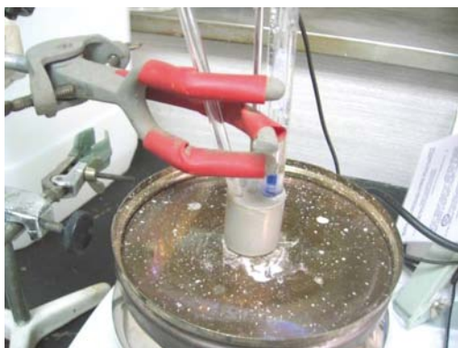
Figure 3-6. Pore water pH measurement for the routine (ESL) method without filtering under N_2 (optionally Argon) gas with the combination pH electrode and temperature sensor inserted directly in the suspension.
