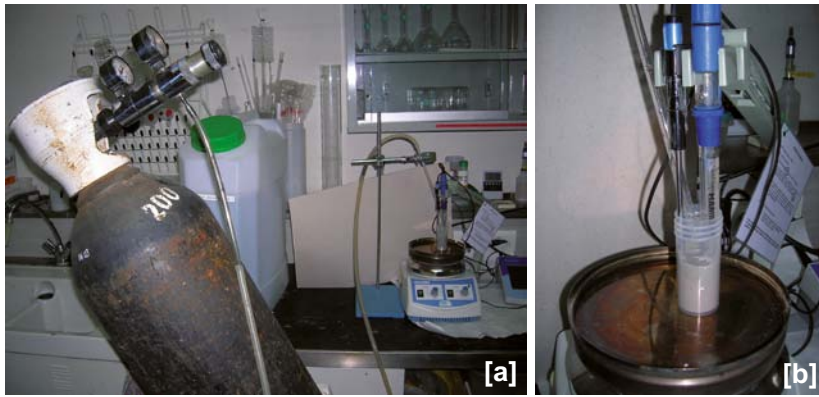
Figure 2-7. pH measurement procedure for the routine (ESL) method without filtering. (a) N_2 (optionally Argon) gas is passed through the head space above the stirred suspension. (b) Detailed view of gas passed through head space and the temperature sensor and combination pH electrode in the suspension.
