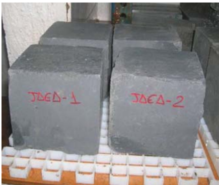
Figure 4-3. Hardened low pH cement paste samples from JAEA as received by CSIC.
