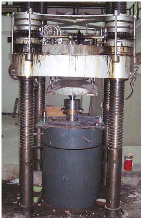
Figure A4-3. Pore expression device placed between the plates of a mechanical press. Photo of CSIC equipment.
