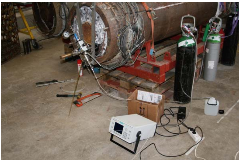
Figure 2-38. Equipment for gas sampling of Heater I.
