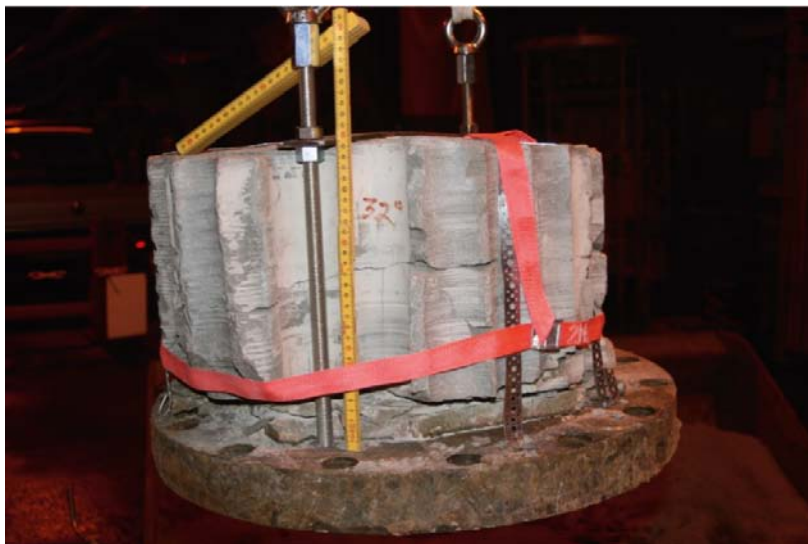
Figure 2-24. Undisturbed bentonite iron interface sample from Cylinder 2. The sample is resting on the lid from Heater I.
