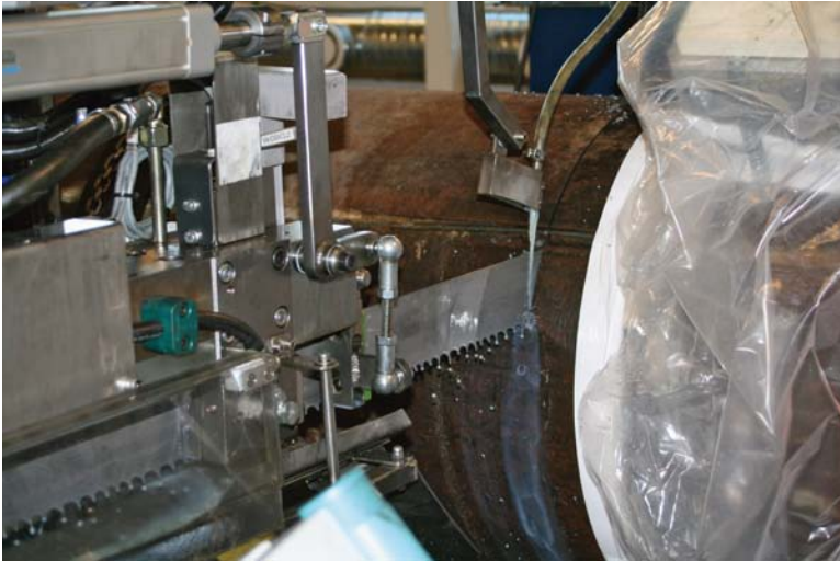
Figure 2-39. Cutting of Heater I. Note the bentonite sample in upper right corner.
