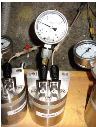
Figure 3-1. Pressure vessels used for extracting pore water and gas from the prototype repository.
