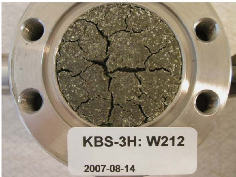
Figure 9-8. Photo taken after lifting the lid but with the specimen still inside the oedometer ring. (Specimen W212).
