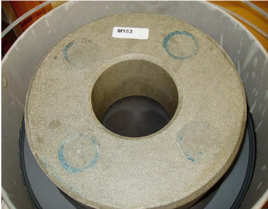
Figure 6-21. Specimen M153 after 3 months. No cracks can be seen on the surface.
