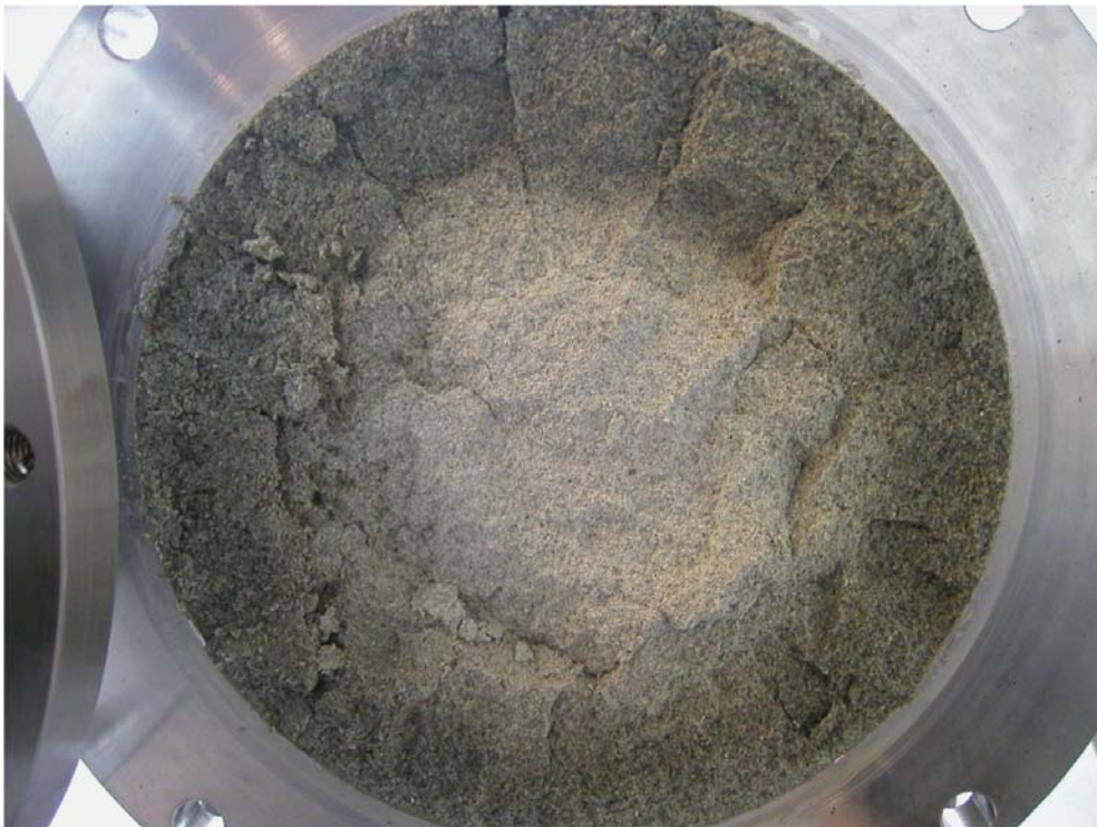
Figure 7-20. Photo taken during dismantling of the test, about 1.5 m from the supercontainer section. The dark ring has a width of 35–40 mm. The water ratio was determined at several locations, see Table 7-5.
