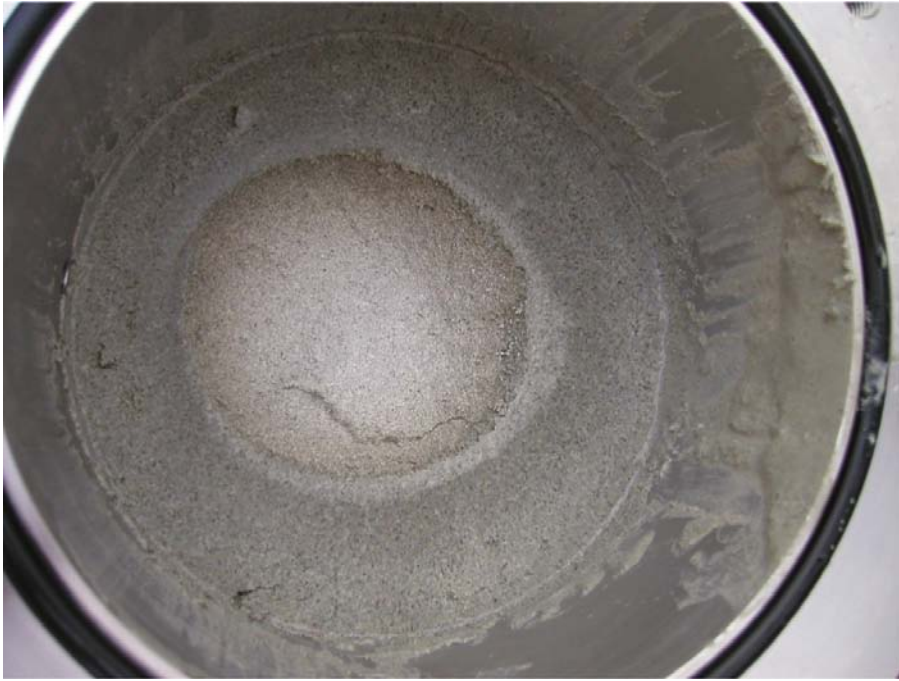
Figure 7-19. The surface just inside the supercontainer dummy. The outer ring-shaped “active surface” can be clearly identified.
