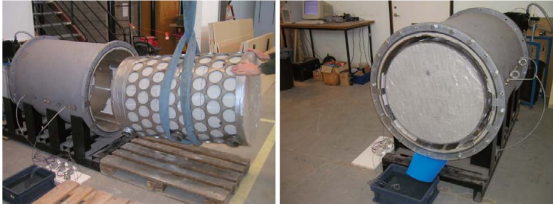
Figure 9-17. Installation of supercontainer simulator. (Left: The open end of the supercontainer was covered with plastic to minimize atmospheric interactions. Right: Plexiglas lids mounted in the ends to allow visual monitoring of bentonite block behaviour.
