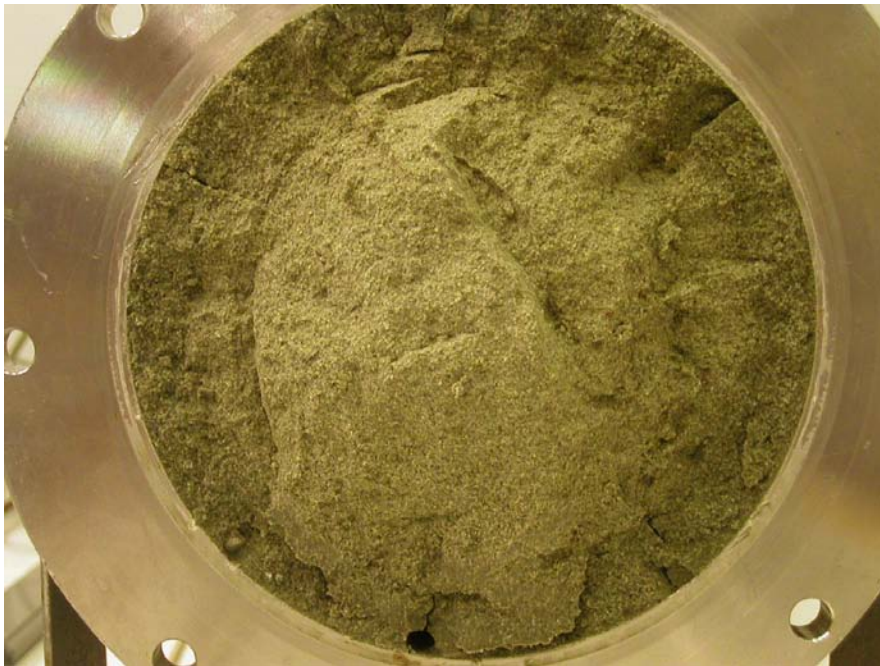
Figure B17-3. Cut about 1.5 m from the super container. The remaining hole from the drainage tube can still be seen.
