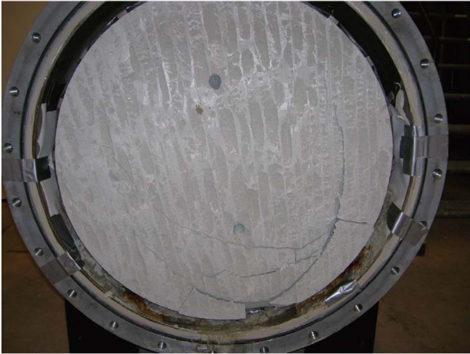
Figure 9-25. Cracks present on the end of the supercontainer after two weeks' exposure to high relative humidity.
