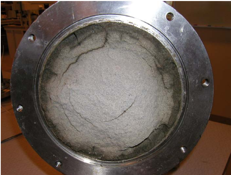
Figure B6-3. Picture from the middle of the sample about 0.5m from the super container side. The water ratio in the outermost 10 mm varied between 40-49% (four samples in different directions).
