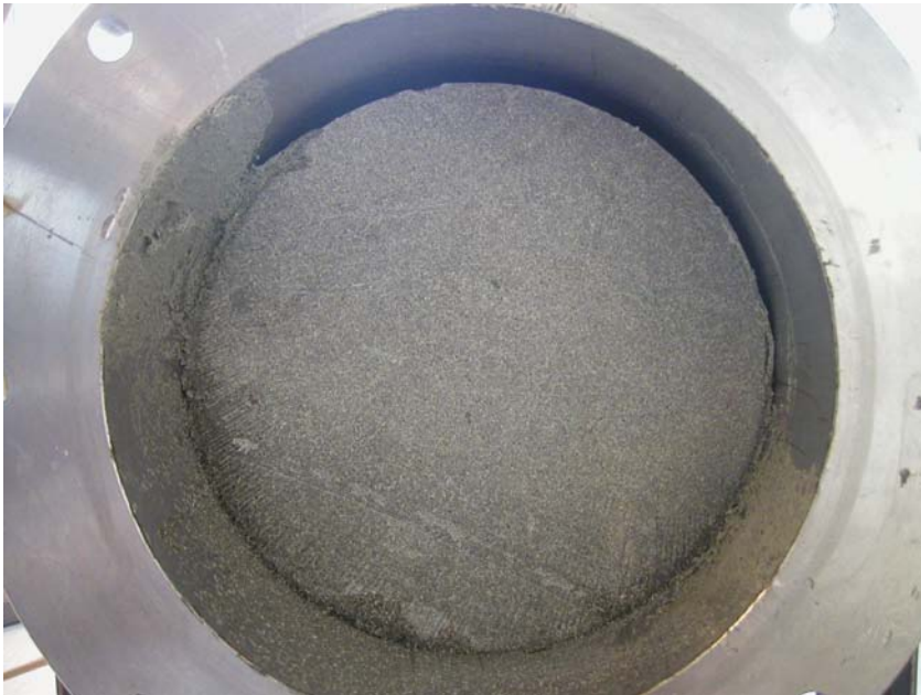
Figure B18-3. Picture showing a distance block about 0.5m from the super container. Only a part of the slot was filled with water due to the fact that the bentonite closest to the super container swelled and sealed very fast and the water had no access to the slot volume inside. When the water pressure ramp was applied the bentonite could not withstand the pressure.
