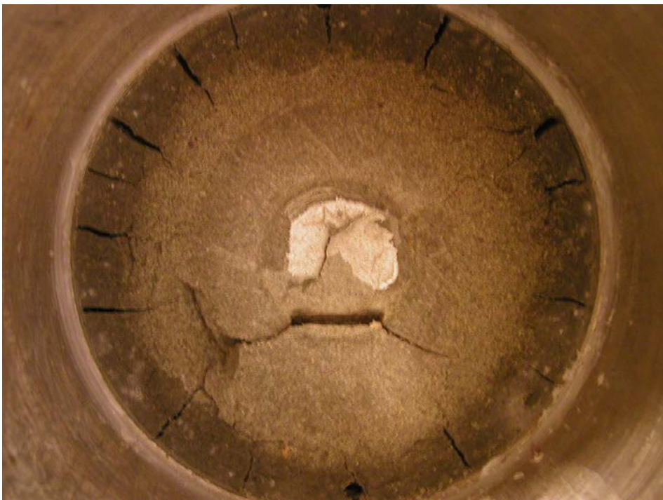
Figure B13-3. Picture showing the distance block after removal of the fixing ring.
