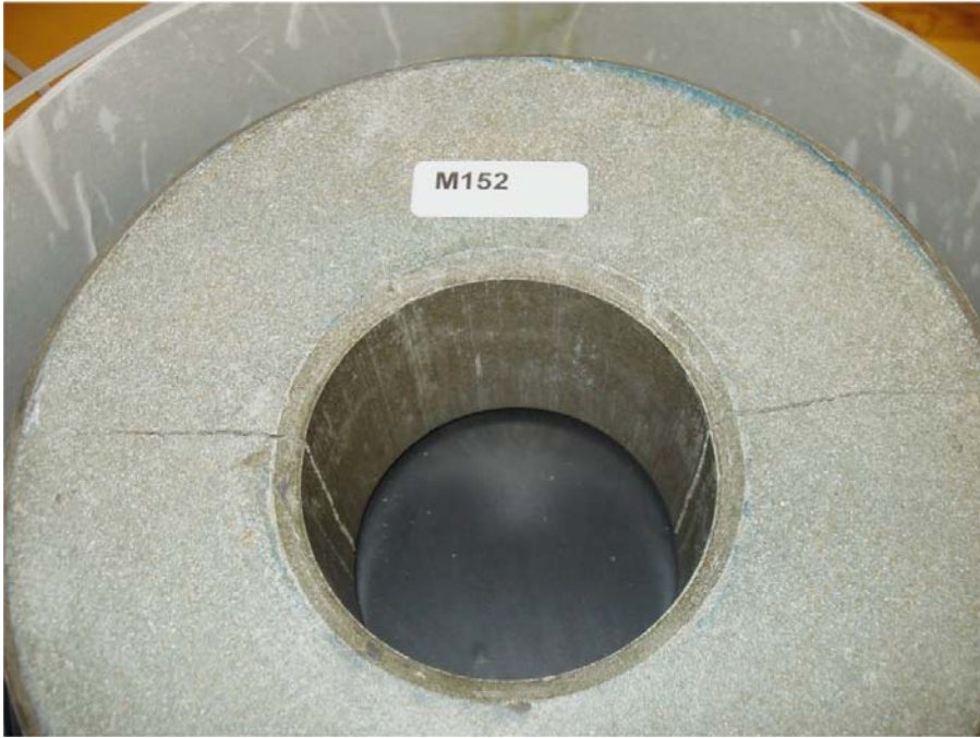
Figure 6-19. Specimen M152 ( w_{ini}=20\% , RH=100\% , gap=45\text{ mm} ) after 7 days.
