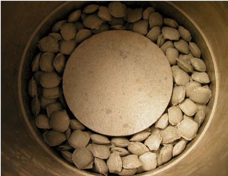
Figure B1-3. Picture from Test 3-1 taken during the preparation of the test showing the central block and the pellets filled slot.
