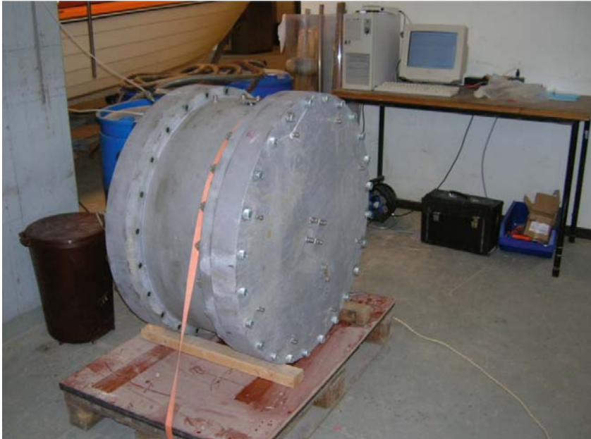
Figure 9-30. Completed installation of radial water uptake test.
