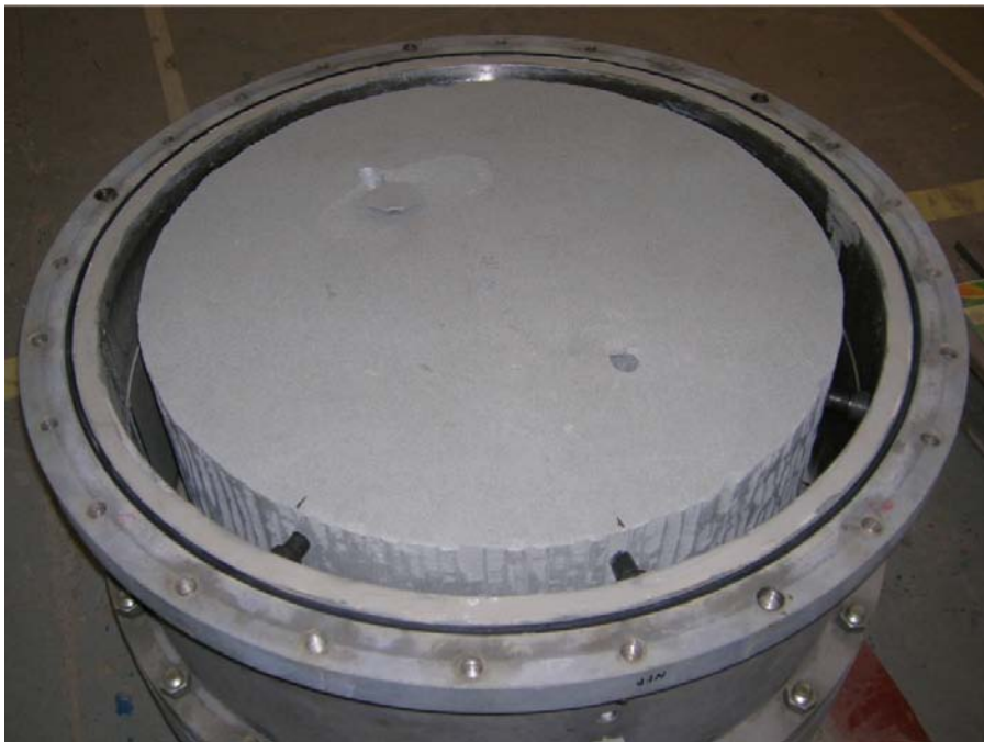
Figure 9-29. Bentonite block centred in the steel "tunnel" through the use of strong bolts.
