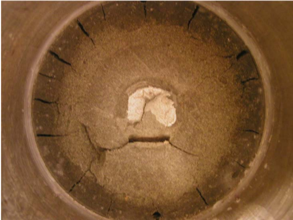
Figure 7-14. Photo showing the outermost distance block after removal of the fixing ring.
