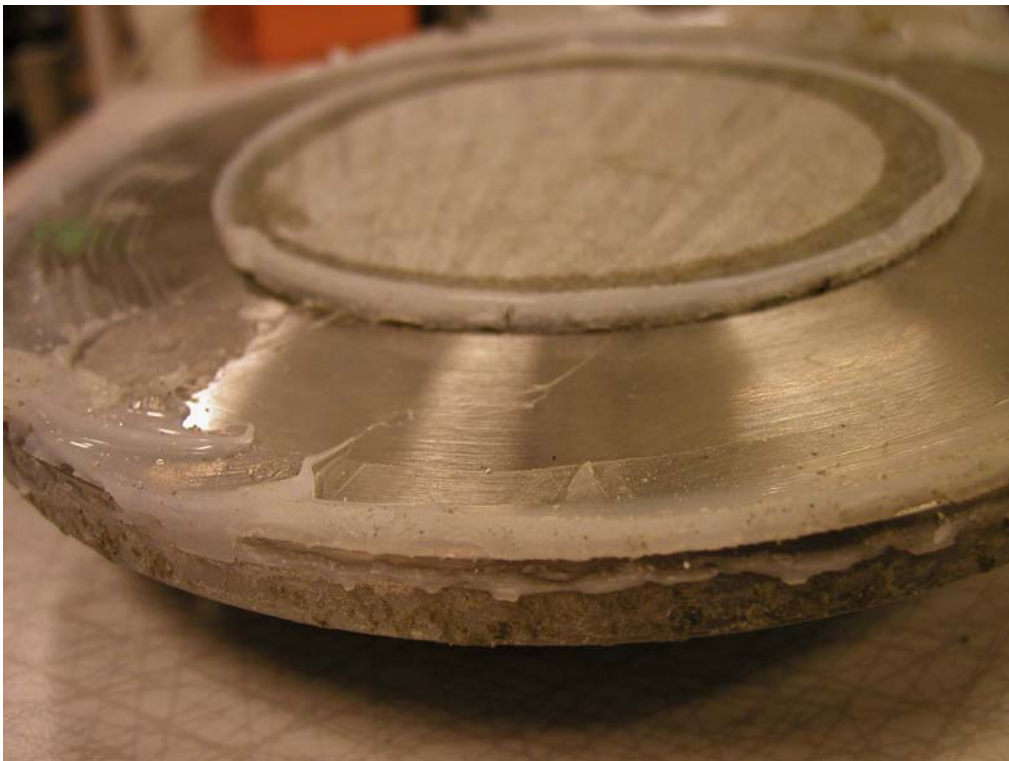
Figure B16-3. Picture showing the fixing ring after dismantling. The bentonite had swelled through the central hole in the fixing ring (totally about 12 mm).
