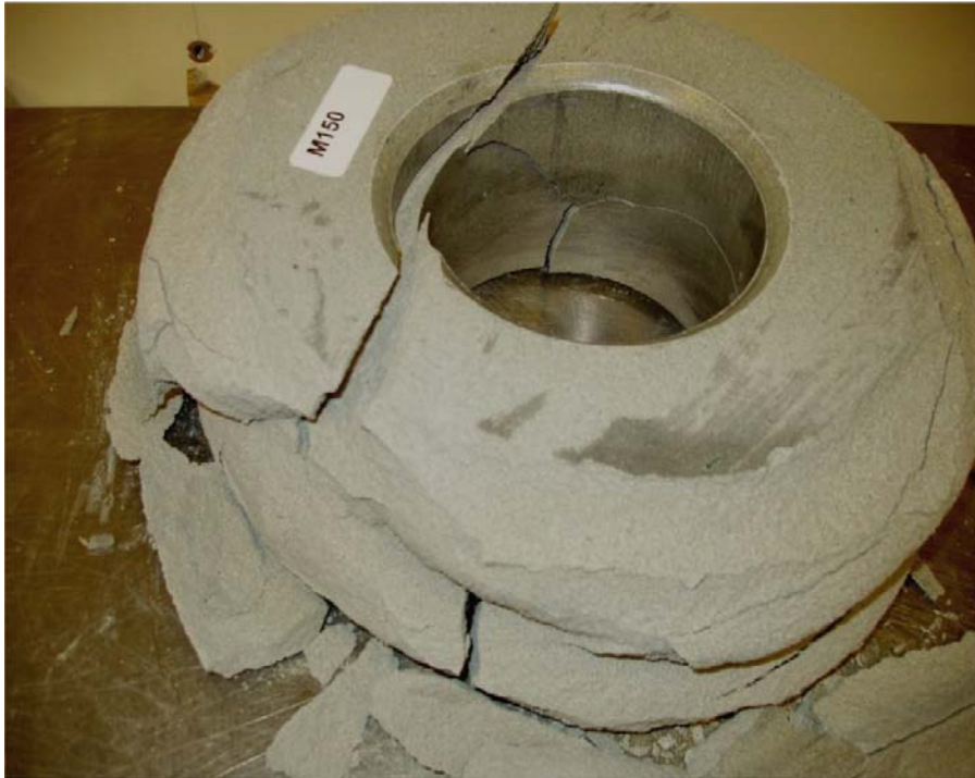
Figure 6-18. Photo showing block specimen M150 ( w_{ini}=13\% , RH=100\% , gap=45 mm) after 8 hours.
