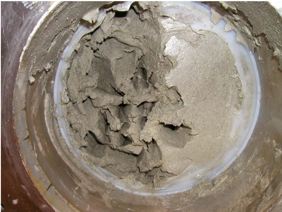
Figure B7-3. Picture showing the surface just inside the dummy simulating the super container. Due to the planned movement of the fixing ring and the followed movement of the distance blocks was the complete area wetted. The depth of the saturated clay was measured to about 6 cm. The water ratio was between 80 % in the centre and up to 90 % in the outermost parts.
