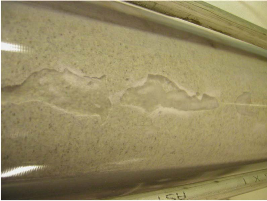
Figure 7-31. Photo taken from above about 0.5 hours after pre-wetting of the outer slot had finished. There are a number of air pockets present on the upper side.
