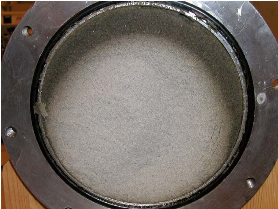
Figure B5-3. Picture from the middle of the sample about 0.5m from the pressure side. The water ratio of the outermost cm clay at the top was 64 %.
