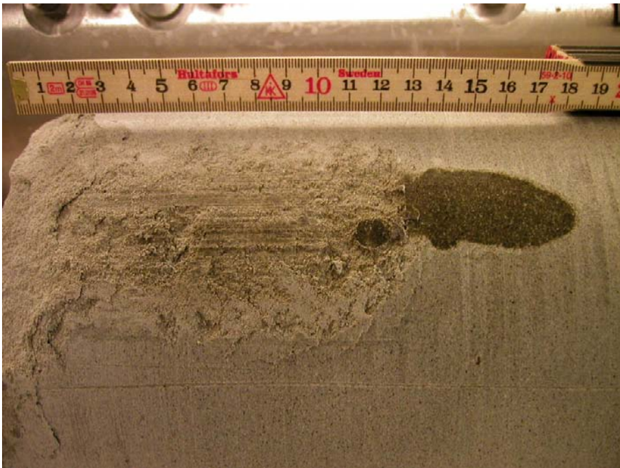
Figure B2-3. Picture showing the outermost half of the test sample after termination of the test. The picture is taken on the bottom side and shows that the depth of the water penetration was about 71 cm (53+18). The cylindrical shaped point that could be seen on the photo is where radial pressure measurement number three has been done.
