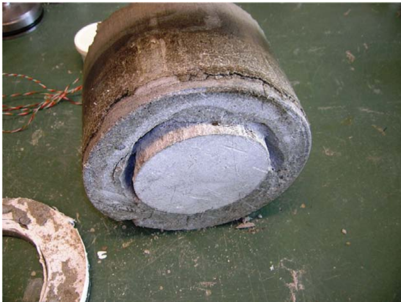
Figure 8-11. Photo showing the bentonite specimen in Test HP404 after dismantling. The central part of the block has been pushed out through the hole in the fixing ring.
