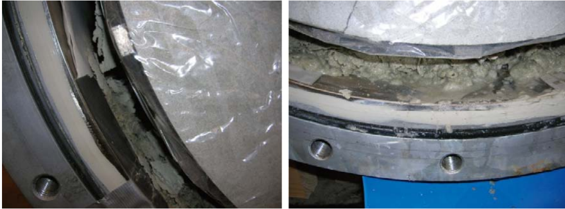
Figure 9-23. View of supercontainer – “tunnel” gap after nine days of testing (note large amount of material that had fallen into the gap).
