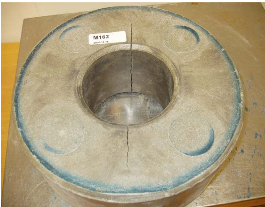
Figure 6-20. Specimen M162 ( w_{ini}=20\% , RH=100\% , gap=65\text{ mm} ) after 3 months. The block was still in one piece but a radial crack had developed after about one month.
