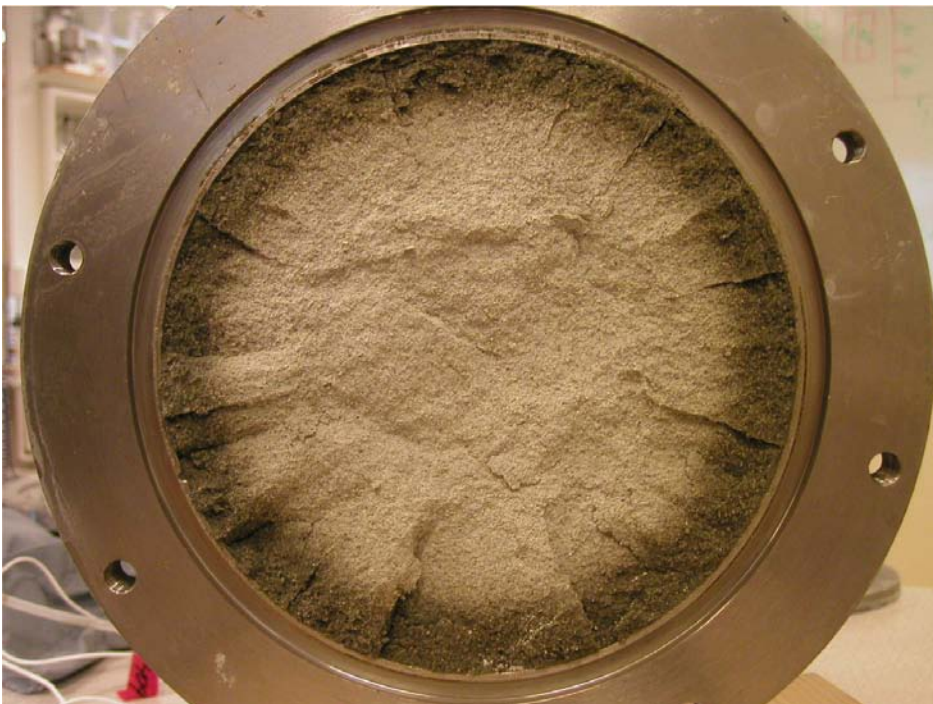
Figure 7-11. Photo of the middle of the specimen about 0.5 m from the supercontainer. The water ratio was determined in several positions with the following results: Outermost 5 mm = 30%, next 5 mm = 29%, next 5 mm = 28%, next 5 mm = 25%, and in the centre = 17%.
