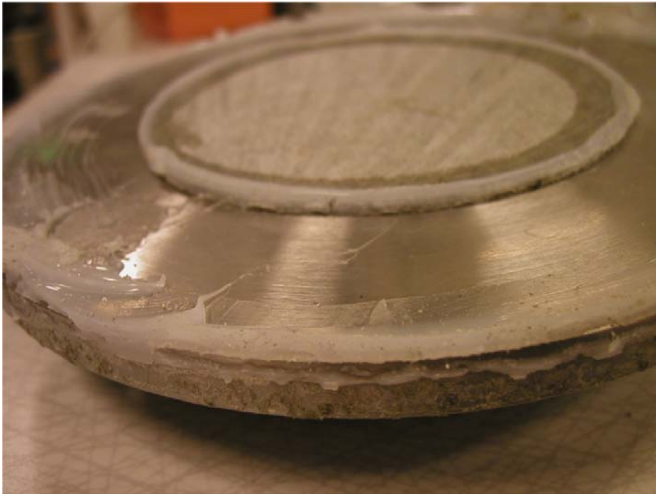
Figure 7-25. Photo showing the fixing ring after termination of the test. The block closest to the ring has been squeezed through the central hole in the steel ring. The total displacement was estimated to be 12 mm.
