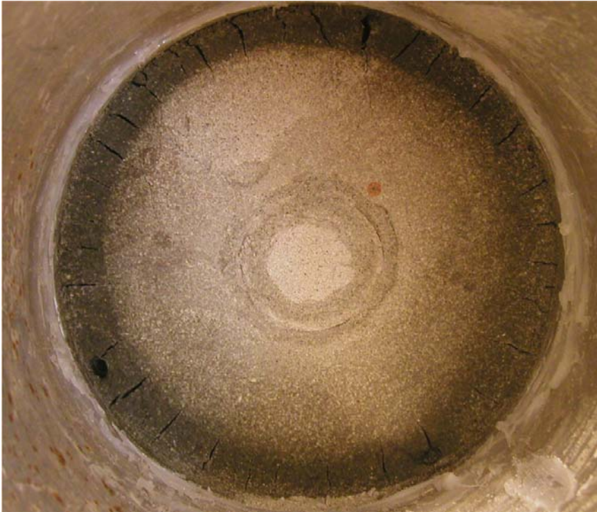
Figure 7-10. Photo showing the outermost distance block just inside the fixing ring. The pre-wetted slot has been filled with swelling bentonite. Since there was no access to additional water from the “rock” after the filling, and the inner parts of the distance block were dry and had a high suction capacity, i.e. affinity for water; there was a redistribution of the available water in the slot. This redistribution resulted in minor cracks occurring in the periphery.
