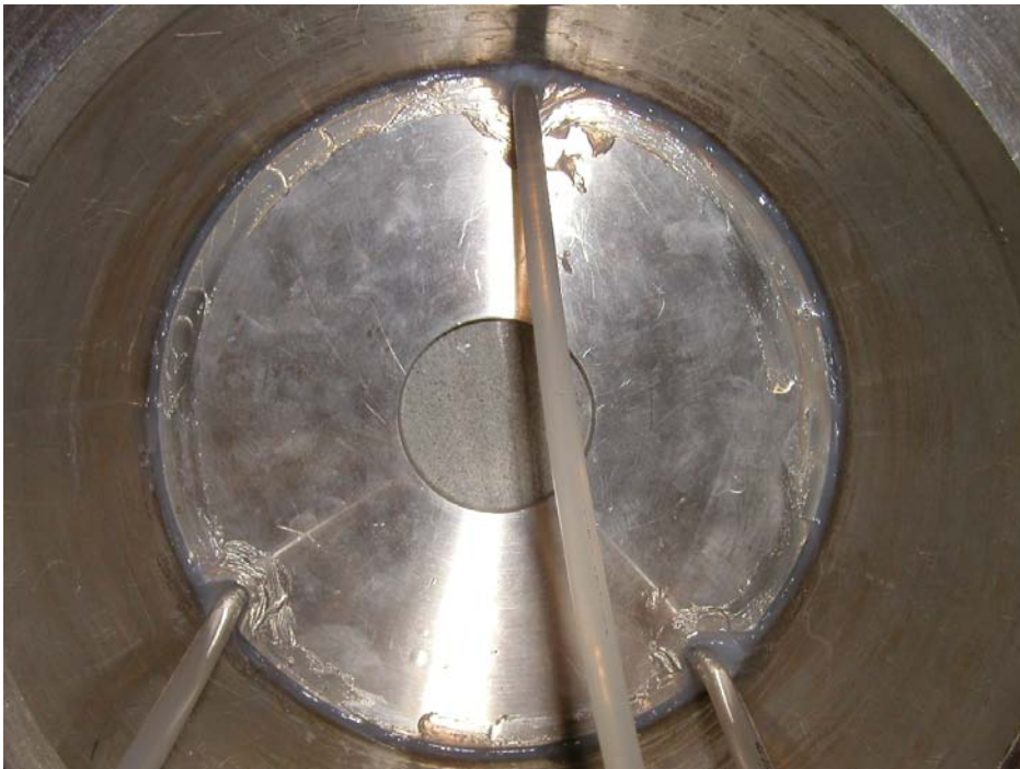
Figure B4-3. Picture showing the outermost part with the fixing ring. The picture shows the tubes used for the pre-filling and de-airing of the volume around the bentonite with water. Silicone was used to seal the slots.
