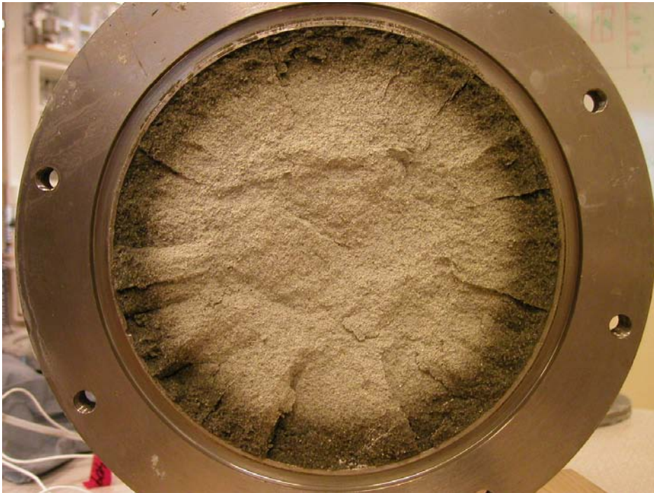
Figure B9-3. Picture from the middle of the sample about 0.5m from the super container. The water ratio was determined in some positions here: Uppermost 5mm=30%, next 5 mm=29%, next 5 mm=28%, next 5 mm=25%, and in the centre=17%
