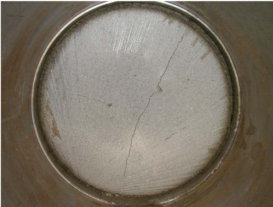
Figure B3-3. Picture showing the outermost part i.e. against the fixing ring. The bentonite has swollen and filled the outer slot but can obviously still not withstand high water pressures.
