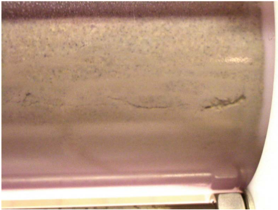
Figure 7-35. Photo taken from side of tube showing the piping channel. For both applied pressure ramps, piping occurred in the same position.
