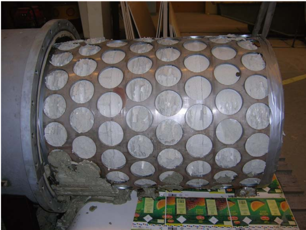
Figure 9-26. Picture taken during the dismantling of the test. The lower part of the bentonite inside the supercontainer had been in direct contact with water.
