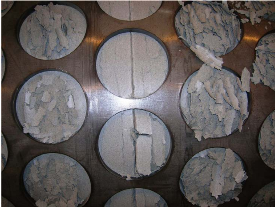
Figure 9-27. Close-up view of the bentonite surface. The cracking of the bentonite surface into flakes was very obvious on all surfaces except in the joints seen in the centre of the photograph.
