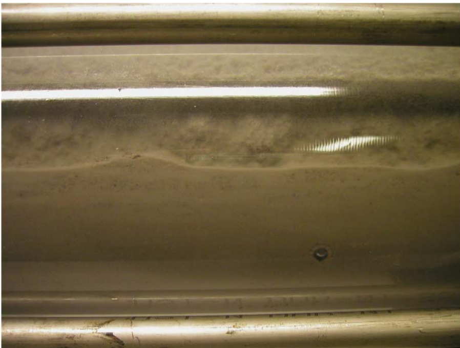
Figure 7-30. Photo taken just after pre-wetting of the outer slot had finished . Bentonite has been discharged from the blocks and settled. Half the slot is still filled with clear water.
