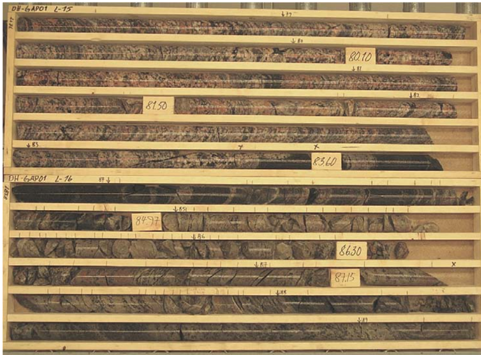
Figure 4-22. Photo showing the main fault zone in DH-GAP01, located in between 84.30 m–89.55 m of borehole length. Photo by Tuomas Pere.
