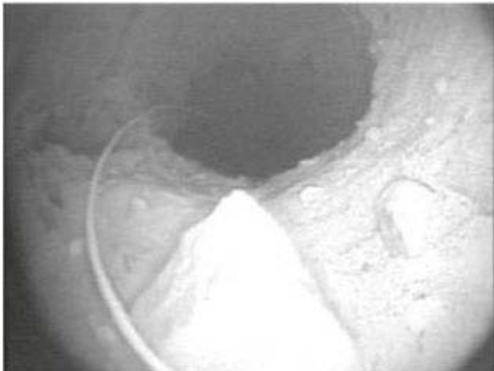
Figure 3-17. Frame grab from borehole video camera showing from about 4 meters above the bed in borehole GL10-2D. The cable for a borehole pressure transducer is visible on left side of image, and has a diameter of a about 4.6 mm. Larger triangular rock protrudes from the borehole wall on bottom side of image. Other rocks are visible within the ice matrix of the borehole wall. Image acquired 25 June, 2010.
