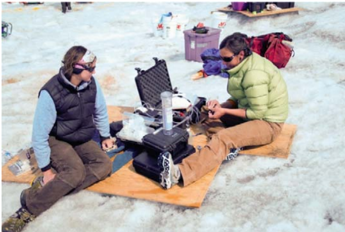
Figure 3-10. Erin Johnson and Claire Landowski measure radon decay in a water sample collected from the bed of the ice sheet. Photo by Joel Harper.
