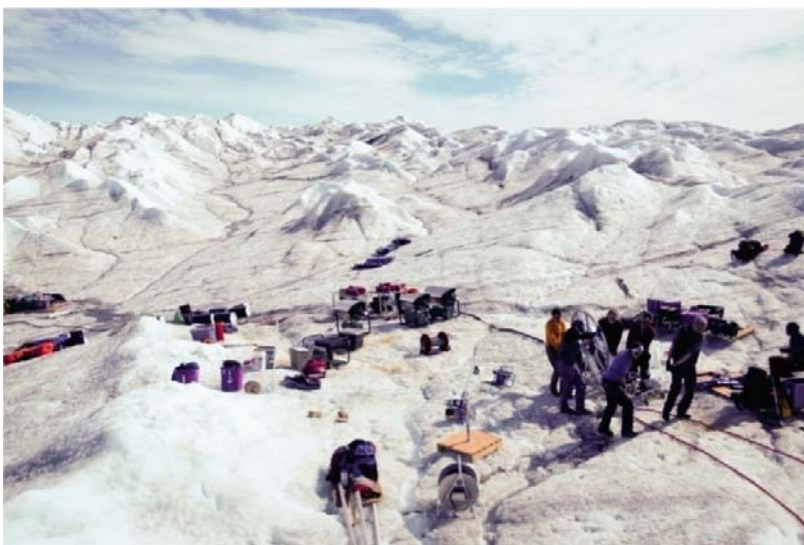
Figure 3-7. The drilling tower can be moved short distances by human power. Here, six persons manually move the drill tower 50 m over rough terrain. Photo by Joel Harper.
