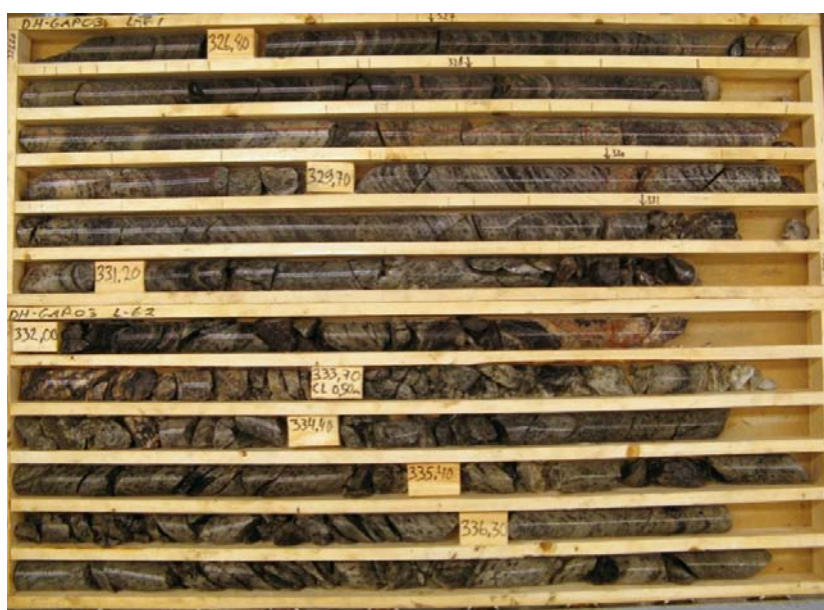
Figure 4-42. Photo showing part of the main fault zone in DH-GAP03, located in between 326.87 m–341.20 m of borehole length. Photo by Tuomas Pere.
