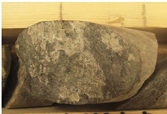
Figure 4-24. Thin white calcite coating on a sheared (chlorite bearing) fracture surface (DH-GAP03, 139.42 m). Photo by Jon Engström.
