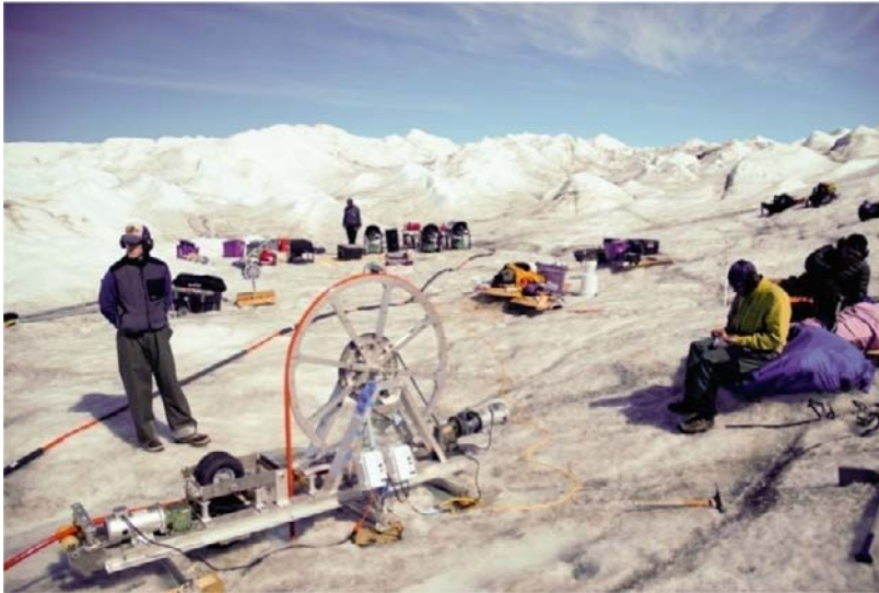
Figure 3-6. Toby Meierbachtol and Chris Cox work next to the newly designed and fabricated drilling tower. The power plant for the drill is visible in the background. All equipment can be moved in 4 helicopter nets weighing 700 kg each (minus fuel). The equipment is easily setup for drilling by a small crew in one half-day, and can be operated with a crew of four persons. Total time for drilling a 700 m borehole is about 7 hours. Photo by Joel Harper
