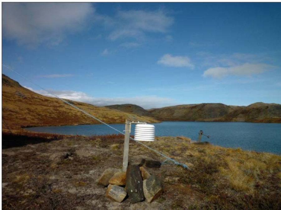
Figure 4-17. Solinst pressure and temperature logger next to DH-GAP01. Photo by Lillemor Claesson Liljedahl.
