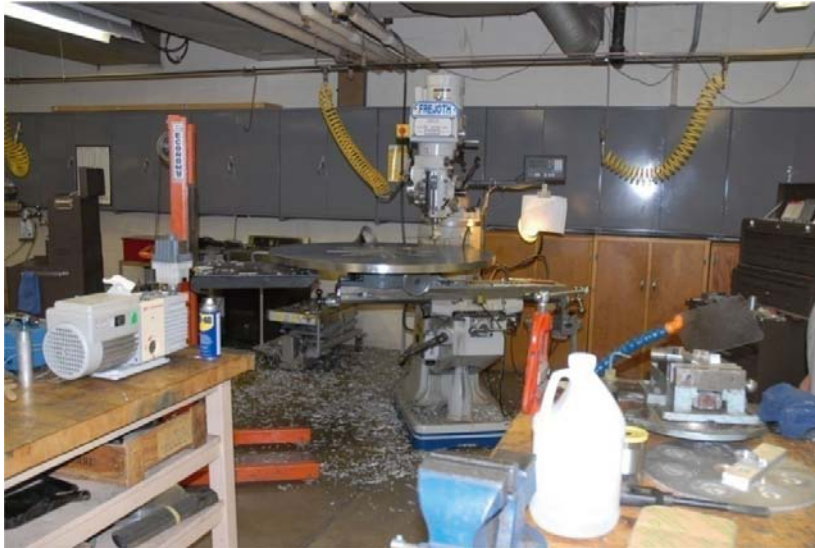
Figure 3-3. The main drive wheel of the Greenland drill, under construction in the University of Wyoming machine shop. The drive wheel is 4ft (1.2 m) in diameter, and was milled from an original 4ft square (1.2 m 2 ) plate of 1.5in (3.8 cm) thick aluminum. Photo by Neil Humphrey.
