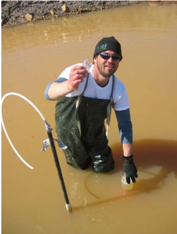
Figure 4-8. Gas sampling method: funnel and mouth of bottle are held underwater as gas displaces water in the glass sampling bottle. Bottle is then capped underwater and kept inverted. Photo by Emily Henkemans.
