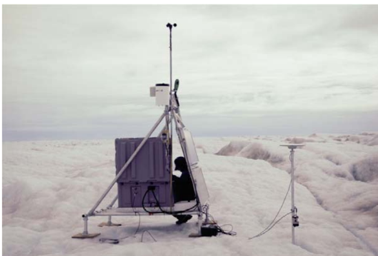
Figure 3-9. Photograph of GPS/meteorological installation. Data are stored at 15 sec to 15 minute intervals and will be retrieved in September, 2010, and spring, 2011. Photo by Joel Harper,
