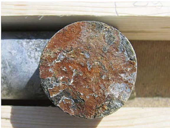
Figure 4-23. Iron oxyhydroxide precipitation on top of calcite infilling in DH-GAP03 at 28.54 m. Photo by Timo Ruskeeniemi.
