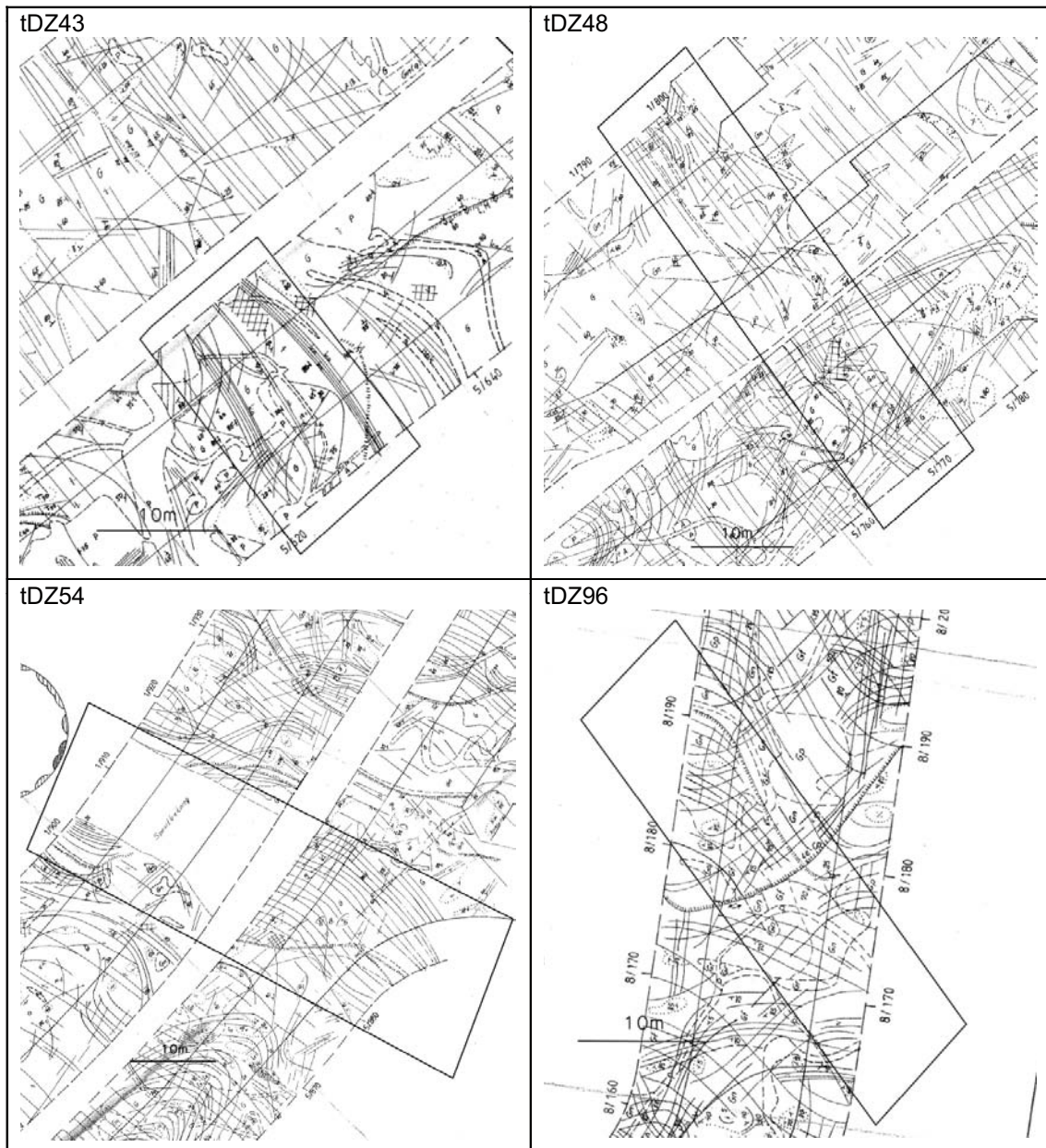
Figure 5-15. Sections of the detailed drawings from /Christiansson and Bolvete 1987/, illustrating the structural relationship for tDZ43 (drawing –07), tDZ48 (drawing –08), tDZ54 (drawing –09) and tDZ96 (drawing –16). The general location of the tDZ's of interest lie within the tunnel sections marked by open rhombs. North is up in all four sections and scale is given by the tunnel chainage. For legend see Figure 3-2.
