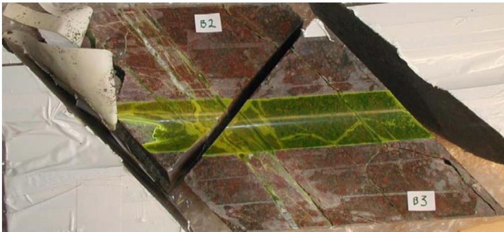
Figure 5-22. This figure is similar to Figure 5-21, but the samples (B2 and B3 from borehole KA2423A03) are rotated such that the cut surfaces are seen. The trace of the 76 mm injection hole may be noted in the centre of the photograph (light green epoxy). (Vertical up direction is normal to the image, directed inwards.)
