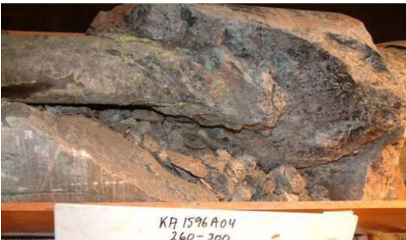
Figure 5-20. KA1596A04. Zone with fault gouge, partially impregnated with epoxy at L=1.9–3.0 metres. No epoxy seen on cylindrical surface of the overcore. Centimetre-sized breccia pieces seen in the lower part of the picture (centre).
