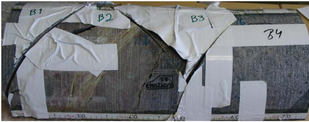
Figure 5-21. The core was cut along the core axis into two halves. Only one half (upper half) was used in the current study. This image shows samples B1, B2, B3 and B4 from borehole KA2423A03. The left side of the core is positioned closest to the tunnel (borehole collar).
