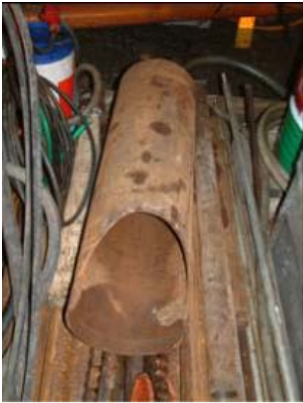
Figure 5-4. Core recovery tool.
