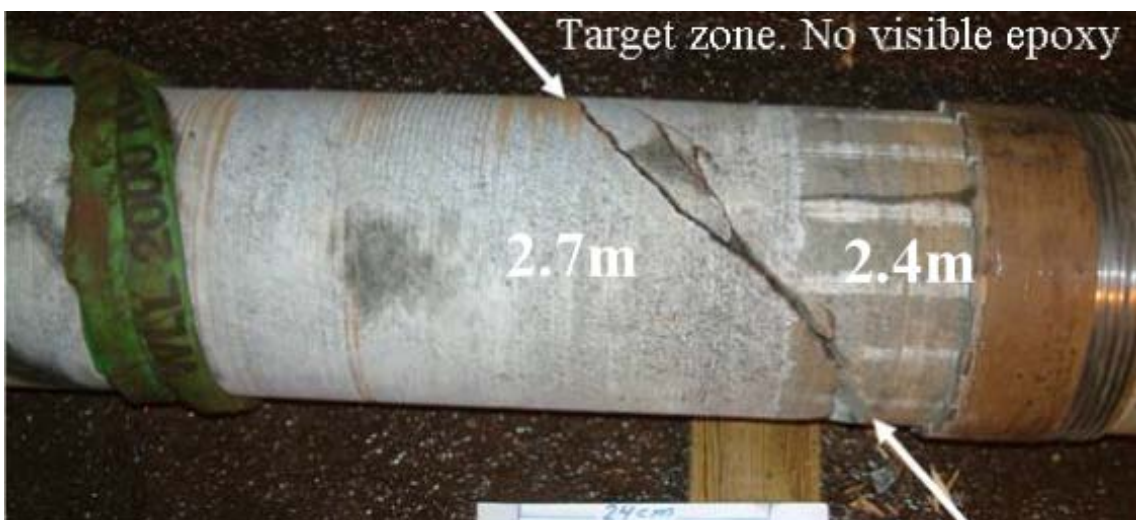
Figure 5-10. KA2169A01. Recovered core with target zone at L=2.5 metres, with no visible epoxy. Hidden under the drill bit (at far right) are epoxy-filled fractures at L=2.10–2.35 metres (cf. Figure 5-11).
