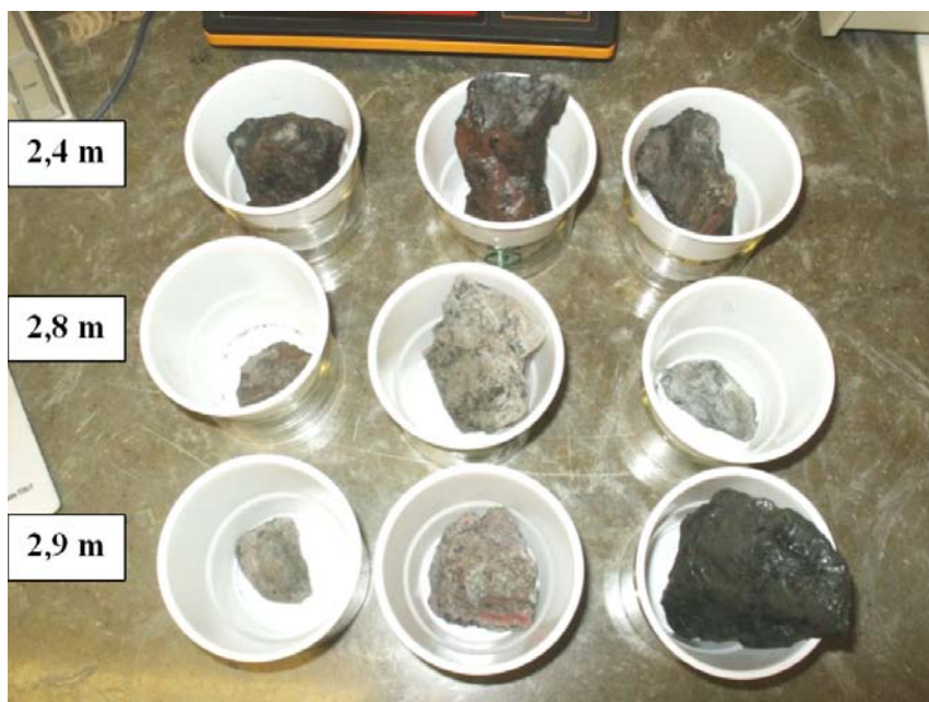
Figure 6-1. Photographs of fault gouge samples (wet state) from the overcore of borehole KA1596A04. Samples denoted A1–A3 (L=2.4m), A4–A6 (L=2.8m), cf. Table 6-1.
