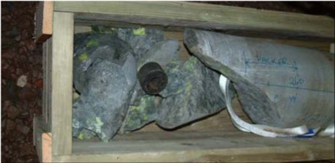
Figure 5-13. KA2169A02. Epoxy patches on fracture surfaces of recovered core segments.
