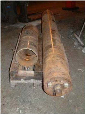
Figure 5-1. 300 mm core barrels with space for 0.76 m and 2.25 m core length, respectively. Scale bar on top of leftmost barrel is 2 m.
