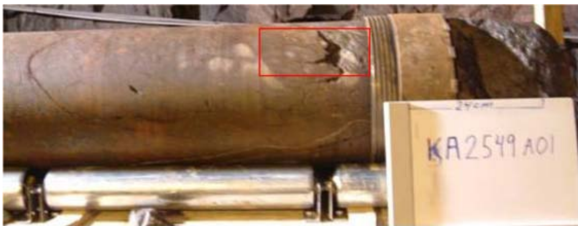
Figure 5-7. KA2549A01. Recovered core with target zone close to metal core bit, and outline (red) of area shown enlarged in Figure 5-8.
