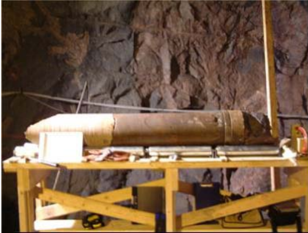
Figure 5-6. Core logging table with rotating cylindrical supports.
