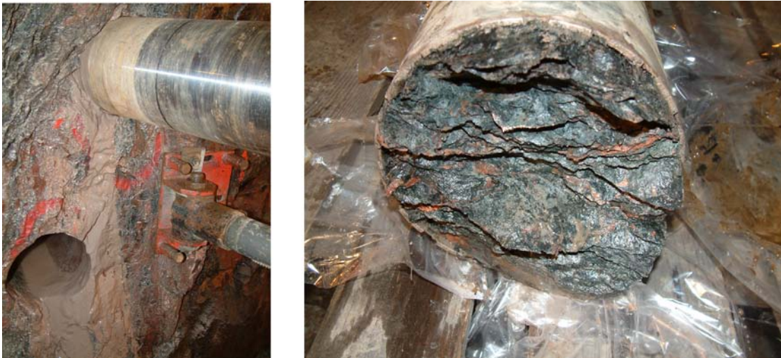
Figure 2-1. Left : Coring with 200 mm barrel in zone NE-2 (zone '1/600'), Right : Example of resulting core.
