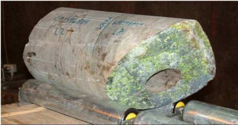
Figure 5-19. KA1596A04. Recovered core with epoxy at L=1.9 metres with face of epoxy impregnated fracture (0°/63°) at L=1.9 metres.
