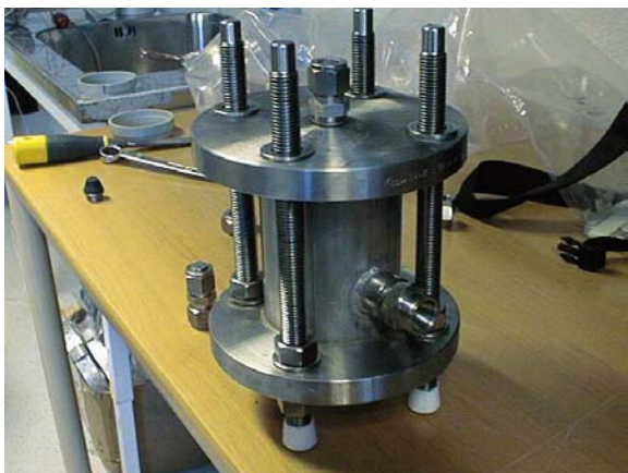
Figure 2-3. Photo of the steel cylinder used to contain the bentonite under its swelling pressure.
