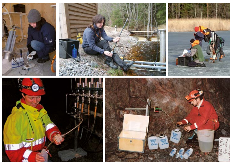
Figure A3-15. Top row: hydrochemical field sampling and analysis during the site investigation at Forsmark in, from left, a deep borehole, a brook and a lake. Bottom row: groundwater sampling in underground environment (Äspö HRL).
