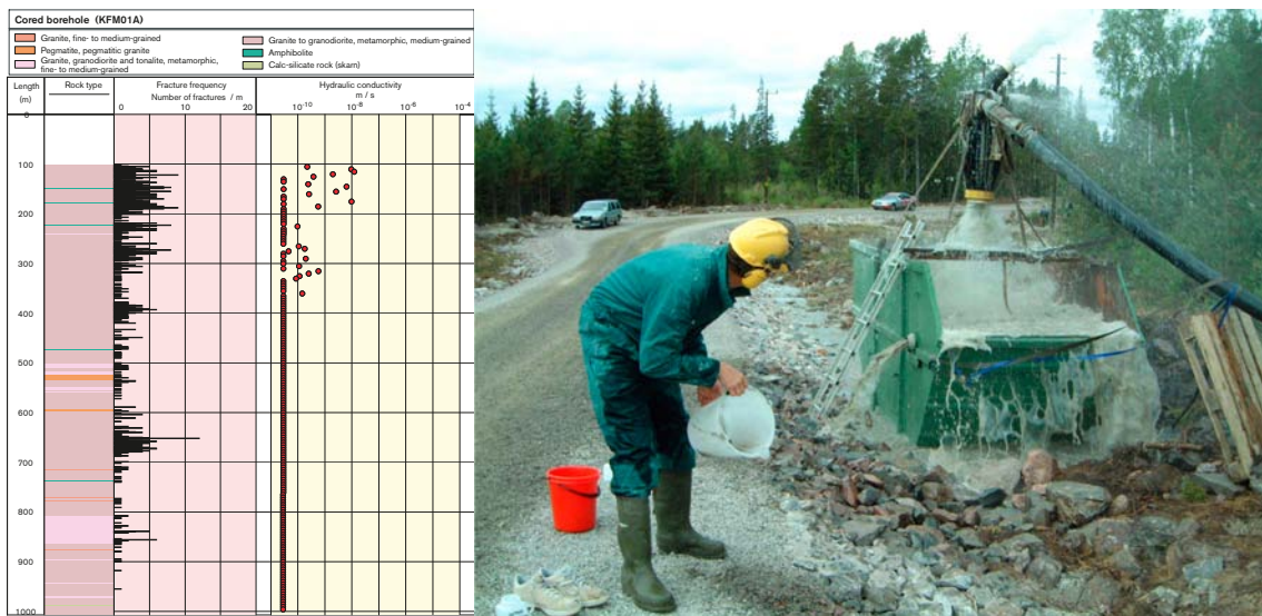
Figure A3-14. Illustration of the contrast in hydraulic conductivity between the shallower and deeper parts of the bedrock within the candidate area at Forsmark for the final repository. At left: chart with rock type and fracture distribution as well as hydraulic conductivity along a 1,000 m long, nearly vertical cored borehole in the central part of the candidate area. Hydraulic conductivity lies at or below the lower measurement limit of the measurement instrument from about 350 m to 1,000 m, while it exhibits a number of high values down to about 200 m. The hydraulic conductivity in the Section 0–100 m, which was percussion-drilled to a large diameter, was determined by an alternative measurement method (capacity measurement at maximum drawdown) and proved to be very high (cf. figure at right). At right: drilling of percussive borehole at Forsmark in the immediate vicinity of the cored borehole illustrated on the left. A water inflow of about 1,000 l/min (at maximum drawdown) was encountered in a short fractured section at about 42–45 m.
