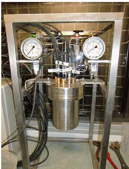
Figure A3-17. SKB's portable measurement instruments for underground measurement of Eh, pH and groundwater temperature. All water hoses are made of PEEK.
