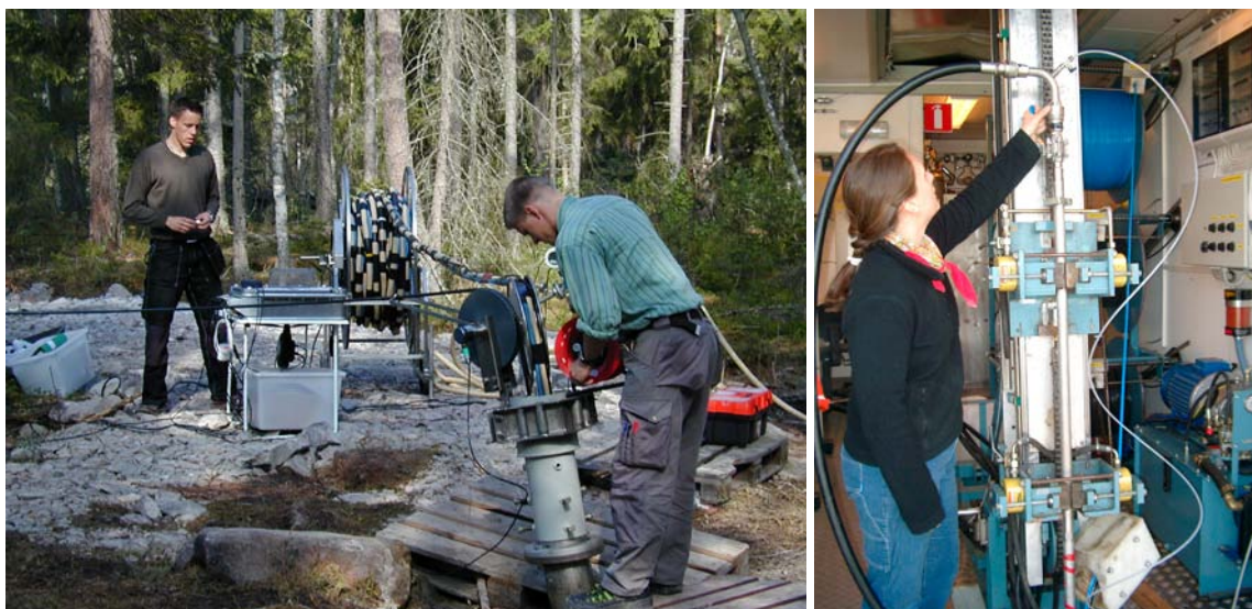
Figure A3-12. Determination of hydraulic parameters in surface boreholes by different methods. At left: pumping test in percussion borehole; at right: injection tests in cored borehole.
