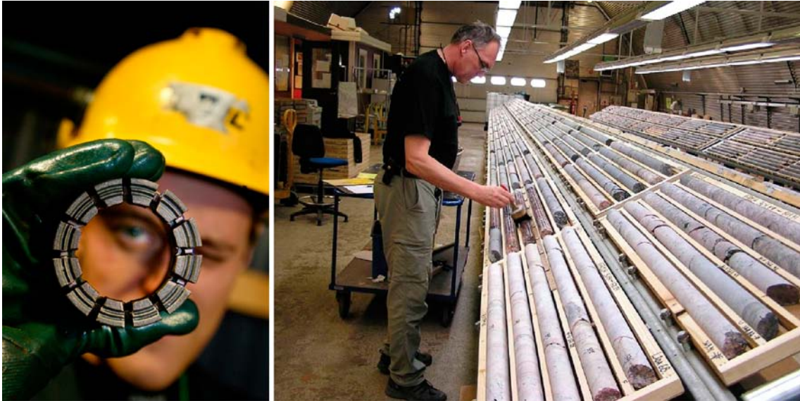
Figure A3-2. At left: core drill bit. At right: mapping of drill cores from a whole cored borehole mounted on a mapping table.
