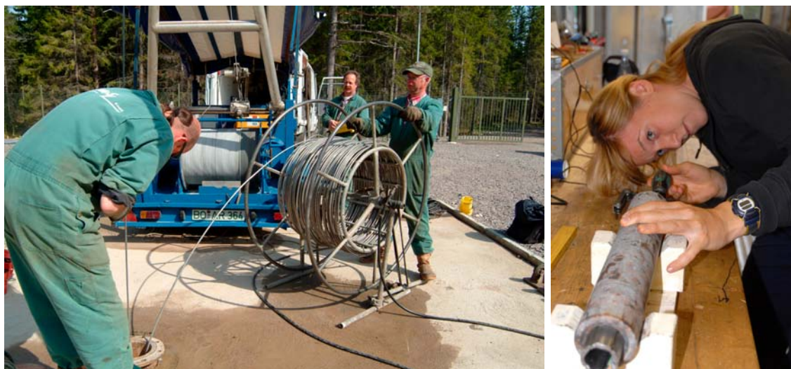
Figure A3-9. Rock stress measurements at Forsmark. At left: lowering of borehole equipment for hydraulic fracturing; at right: study of freed drill core from overcoring measurement.
