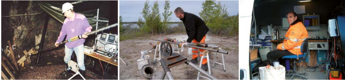
Figure A3-5. Geophysical borehole investigations. From left: 1) BIPS logging in underground hole, 2) conventional geophysical borehole logging in surface borehole and 3) interior from measurement bus for geophysical logging.
