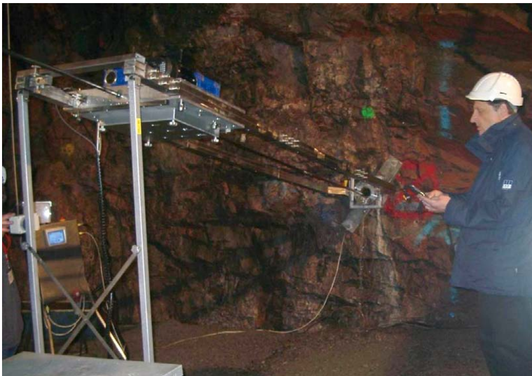
Figure A3-8. Insertion equipment intended for e.g. borehole geophysical equipment in horizontal, subhorizontal and upward-directed underground boreholes.
