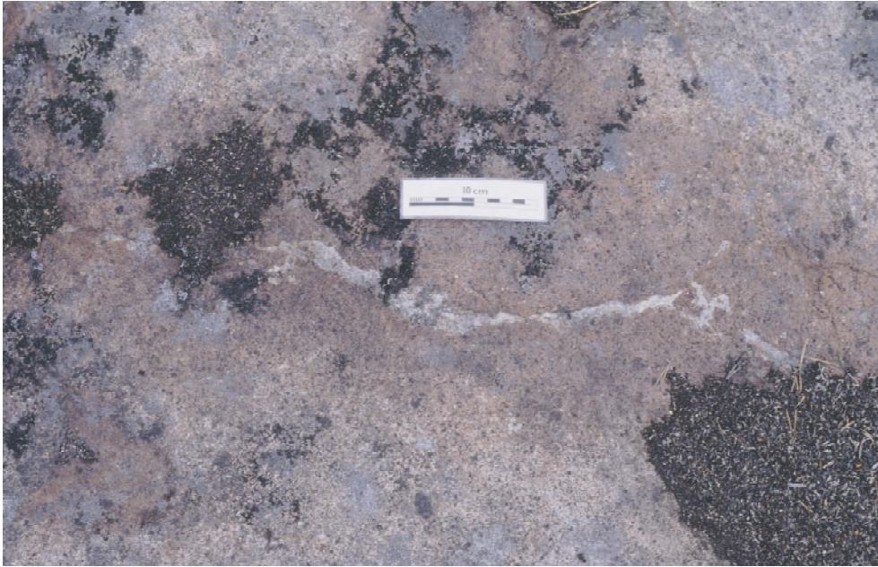
Figure 5-22. Red staining along a sealed fracture in fine-grained dioritoid. The mineral infilling is supposedly dominated by prehnite.
