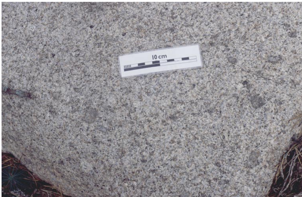
Figure 5-17. Sparsely porphyritic Ävrö granite.
