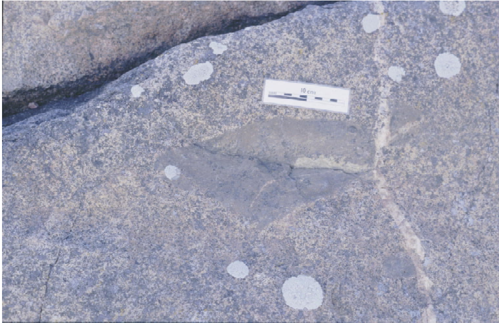
Figure 5-13. Inclusion of fine-grained dioritoid in quartz monzodiorite.
