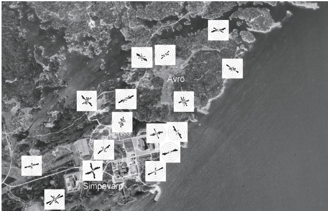
Figure 5-4. Orthophoto with diagrams showing fracture strike and frequency for fractures dipping 45 degrees or more at each outcrop. Note that the frequency scale is different between outcrops.
