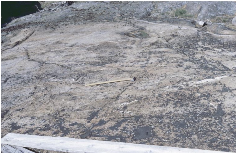
Figure 5-23. Red staining in Ävrö granite.
