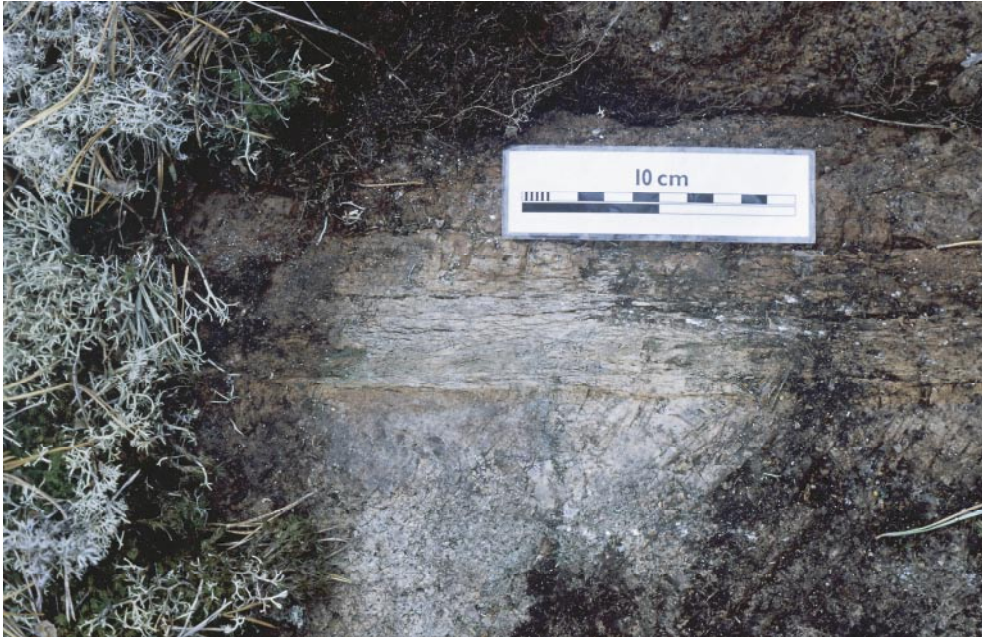
Figure 5-20. Dm-wide, low-grade ductile shear zone in Ävrö granite.
