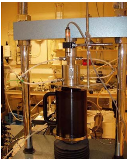
Figure 3-20. A pressure cylinder was used as loading device for application of high load.
