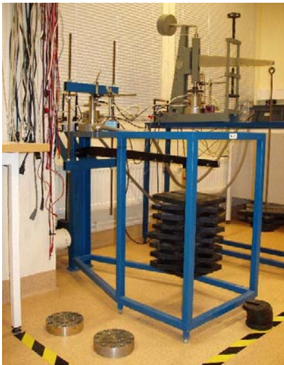
Figure 3-19. Maximal loading applied on one of the loading frames.
