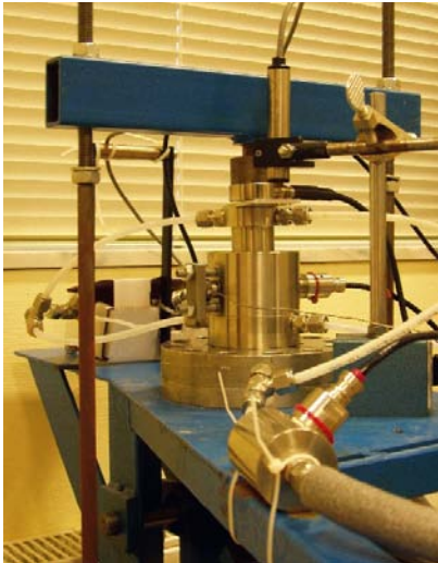
Figure 3-18. Device used for the oedometer tests. The oedometer is equipped with a deformation sensor, a force transducer and an RH sensor.
