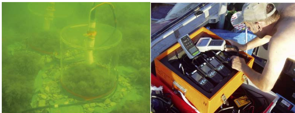
Figure 3-29. Measurements of benthic primary production and respiration in a red algae community in Laxemar-Simpevarp /Borgiel et al. 2006/. Photo: M. Borgiel.
