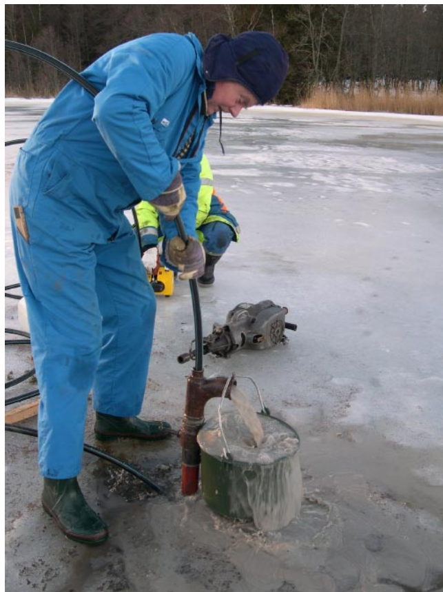
Figure 4-1. Leif Lundholm, Sweco VBB Viak, performed the sampling of till from beneath the lakes by flushing the sediment.
