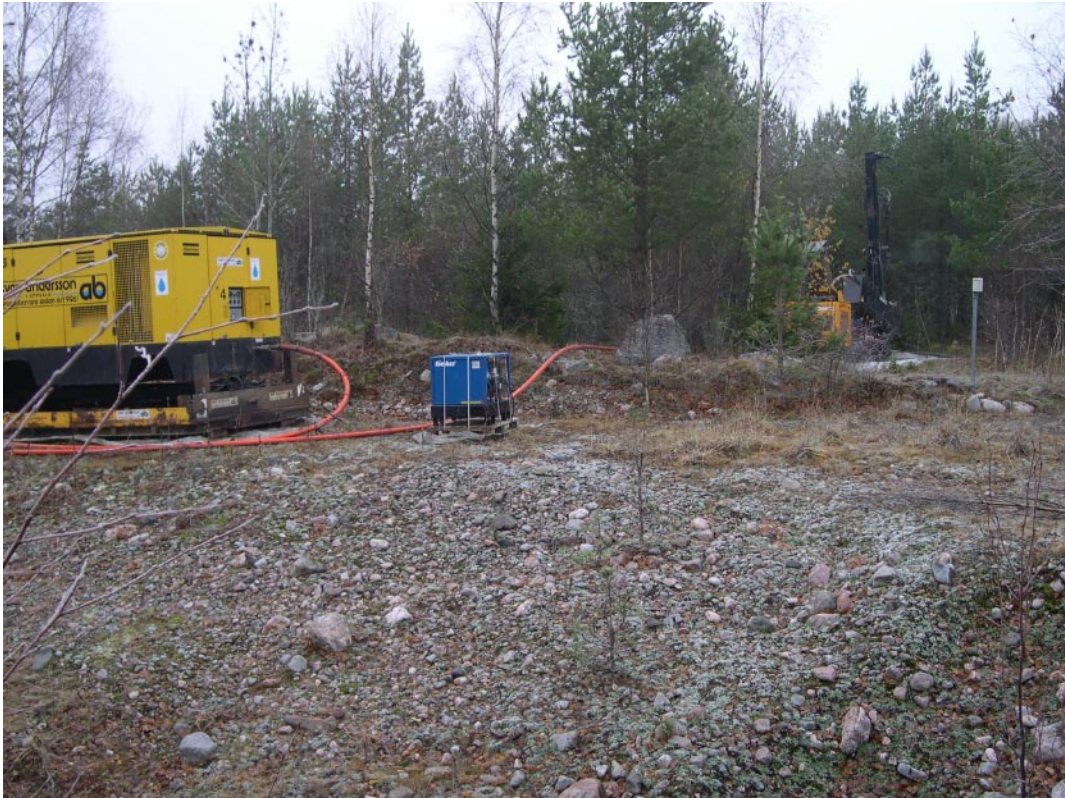
Figure 5-2. Percussion coring at SFM0060 at the Börstilåsen esker. The glaciofluvial sediment was sandy gravel at the surface and coarser gravel further down. The sediment in the foreground (gravel) is exposed in an old gravel-pit.
