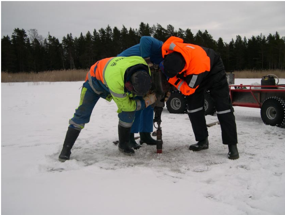
Figure 5-1. Leif Lundholm and Patrick Smützer from Sweco VBB Viak, sampling at Lake Gällsboträsket. At c. 3 m depth, the till was very hard and could not be penetrated without the extra power from Kenneth Åkerström (to the right in the picture).
