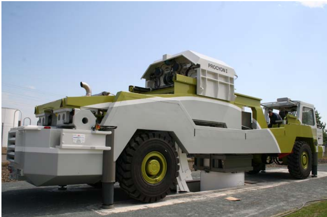
Figure 2-5. Deposition machine for handling of canisters in the final repository.
