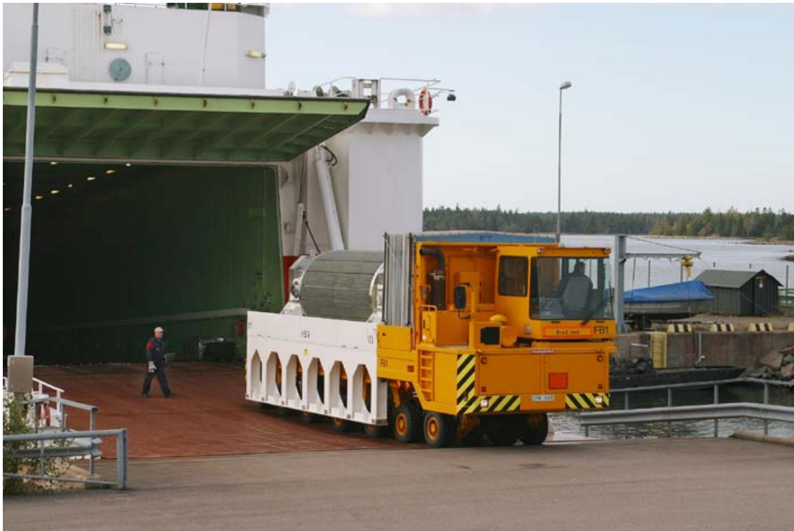
Figure 2-14. Terminal vehicle with transport cask.
