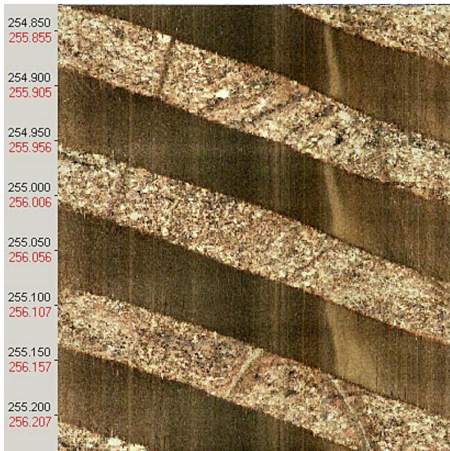
Figure 4-1. BIPS-image from the length interval 255.83–256.24 m of borehole KFM03A, illustrating the distinct spiral pattern of brownish coating at the borehole wall.
