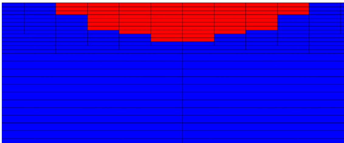
Figure De6-2. Computational grid. At ground level (top) and a section through the stream, where the cells are 0.13·1.0 m (z, y). In the top figure the blue grid marks the sea.
