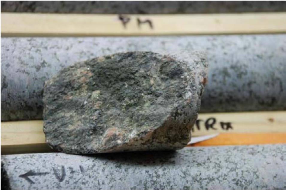
Figure 5-22. Photo of KLX17A (fracture ID: 3497478B0A21F03D) showing a typical Group 6 fracture with clear signs of mineral coating (in this case chlorite, calcite and pyrite). The diameter of the drill cores is 50 mm.
