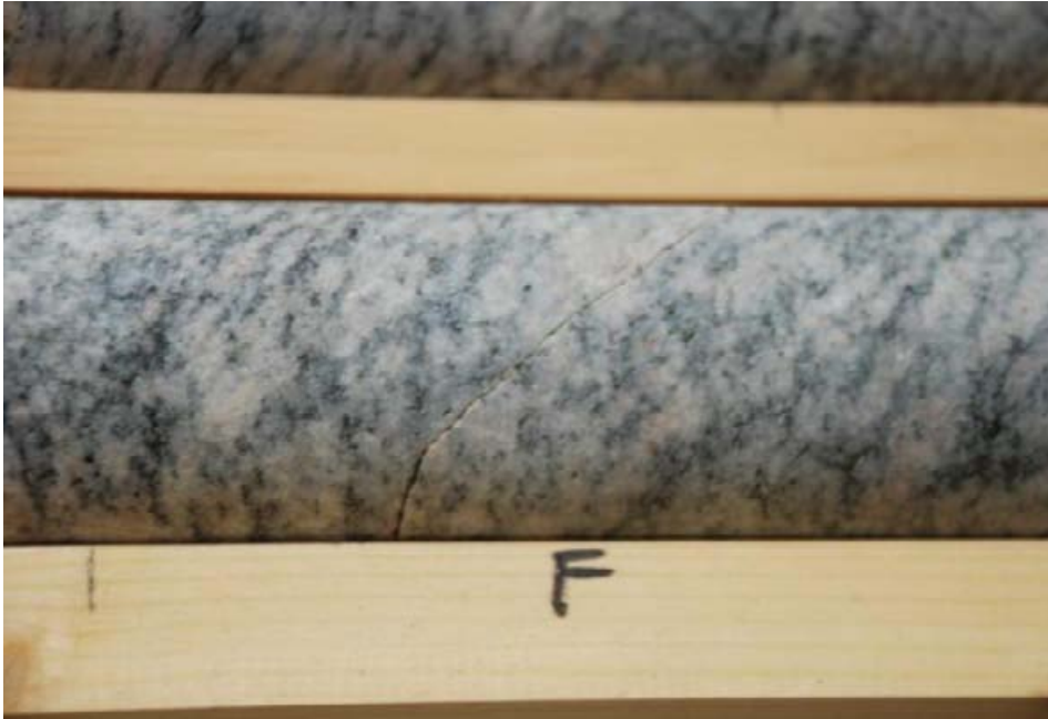
Figure 5-12. Photo of core KFM01D (fracture ID 521142D98F180CA9). F indicates that this break occurred during handling of the core. This fracture is a typical Group 7 fracture; it is not visible in BIPS (see Figure 5-11), and was erroneously logged as an in situ fracture. The diameter of the drill cores is 50 mm.
