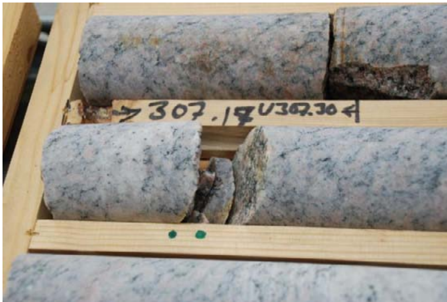
Figure 5-4. Photo of core KFM06A (fracture ID 60D642D98A327BFD). This fracture is a typical Group 1 fracture: it is clearly visible in BIPS, and the missing material in the core coincides with drilling disturbances. The diameter of the drill cores is 50 mm.
