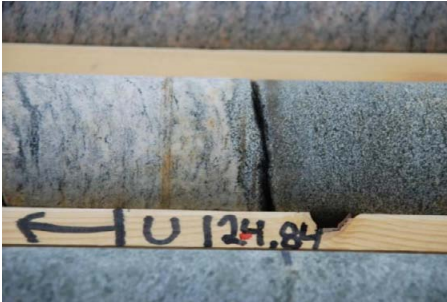
Figure 5-5. Photo of core KFM02A (fracture ID E8D242D98A31E7B6). This fracture is a typical Group 2 fracture, as it coincides with or is affected by drilling disturbances. In this example the fracture coincides with a change in lithology at the uptake of the drill core. The diameter of the drill cores is 50 mm.
