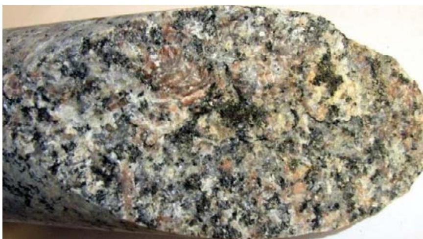
Figure 5-26. Photo of KLX18A (fracture ID: 8098478B0A171FDD) showing a fracture with no visible mineral coating (i.e. a group 5 fracture). Pyrite crystals were observed when the surface was examined using SEM-EDS, see Figure 5-27.
