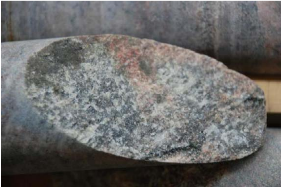
Figure 5-7. Photo of core KFM06C (fracture ID 7C9642D9881B5146). This fracture is a typical Group 4 fracture, with indications of mineral coating but the coating is too thin to distinguish the minerals forming the coating with the unaided eye. This fracture was sampled for further mineralogical analyses. The diameter of the drill cores is 50 mm.
