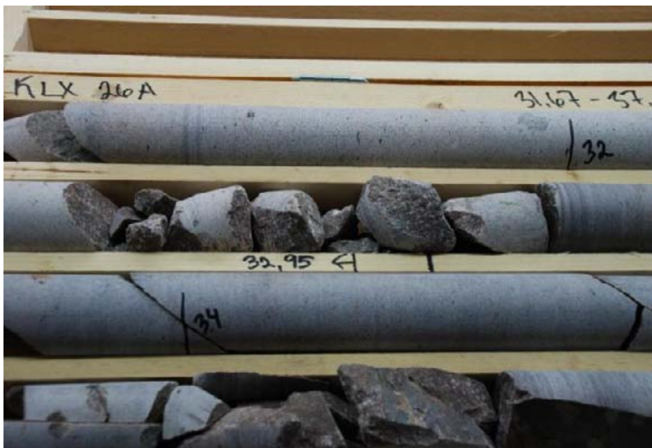
Figure 5-19. Photo of core KLX26A (fracture ID:s C0964B8B0A1080C3; 20964B8B0A1080F4; 40964B8B0A1081A9). This photo shows several fractures typical of Group 2 fractures, where core/fracture and/or material is missing due to drilling disturbances. The diameter of the drill cores is 50 mm.
