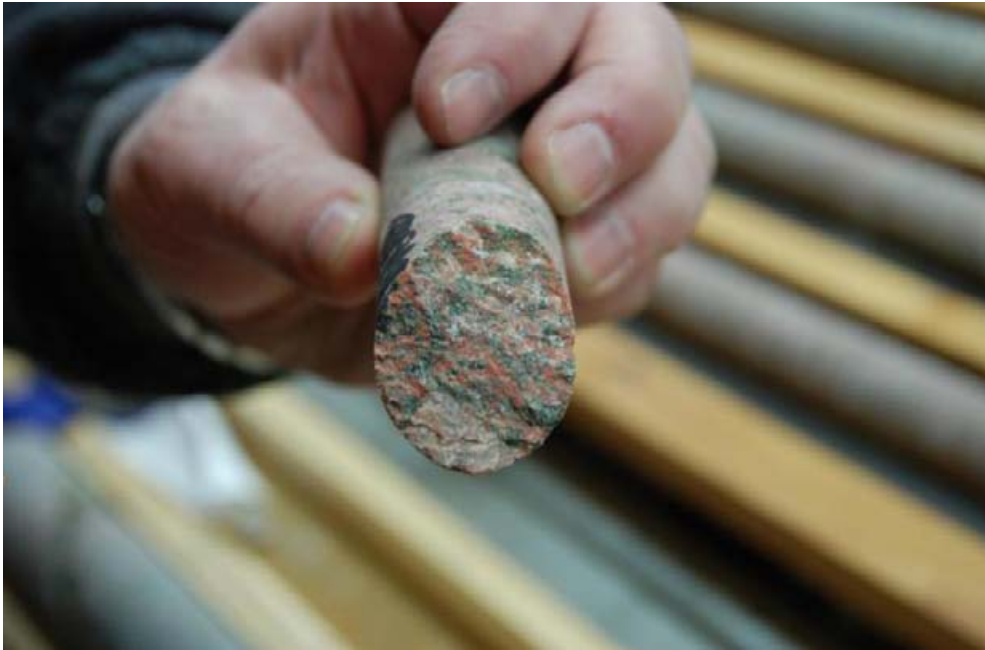
Figure 5-20. Photo of KLX08A (fracture ID: 4CD8438B2B149FB3) showing a Group 4 fracture with indications of mineral coating. The diameter of the drill cores is 50 mm.
