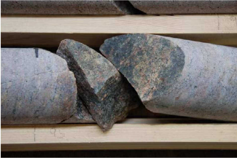
Figure 5-10. Photo of core KFM10A (fracture ID BF5046D98A11738D). This fracture is a typical Group 6 fracture, with clear indications of mineral coating. This fracture was sampled for further mineralogical analyses. The diameter of the drill cores is 50 mm.
