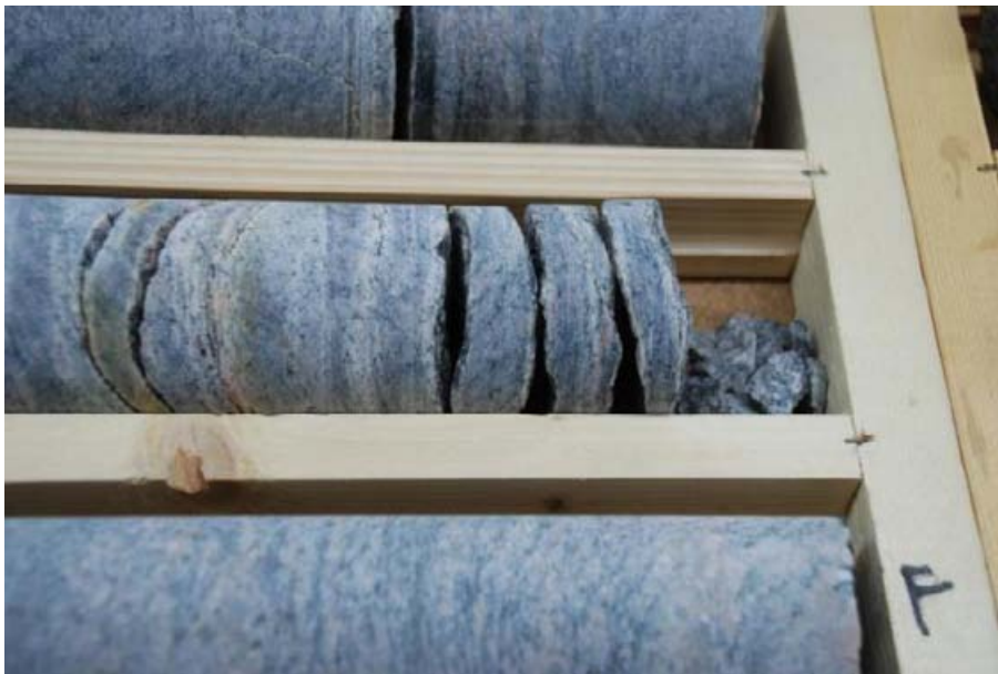
Figure 5-6. Photo of core KFM10A (fracture ID 25D046D98A15B32C). These fractures are typical Group 3 fractures and display strong indications of core dishing. The core dishing appear to coincide with nearby bands of micro-fractures. The diameter of the drill cores is 50 mm.
