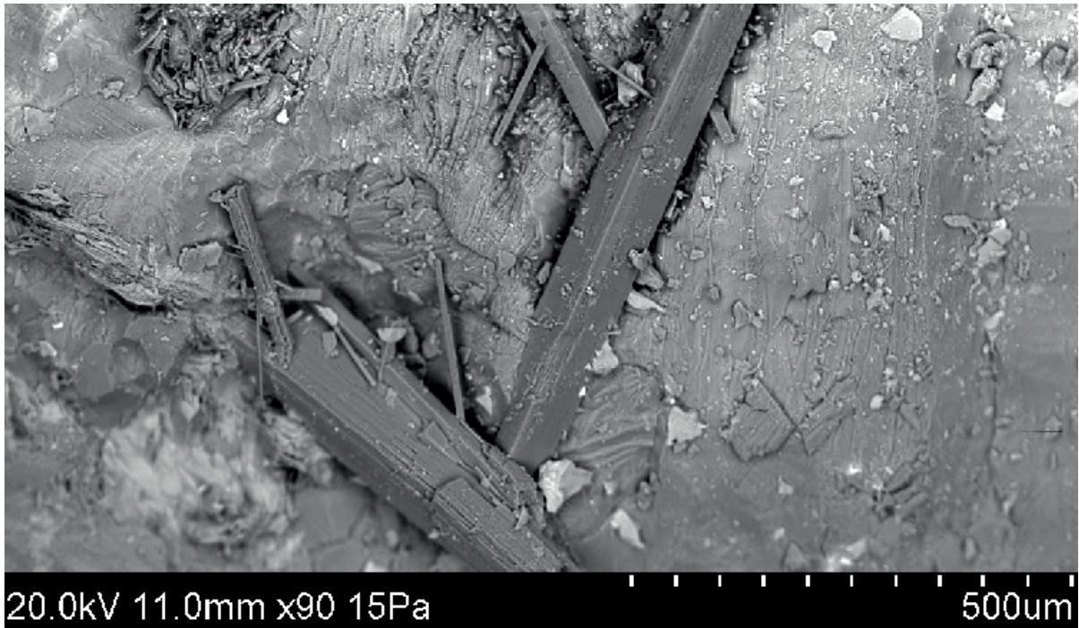
Back-scattered SEM-image of Na-zeolite (euhedral crystals).
