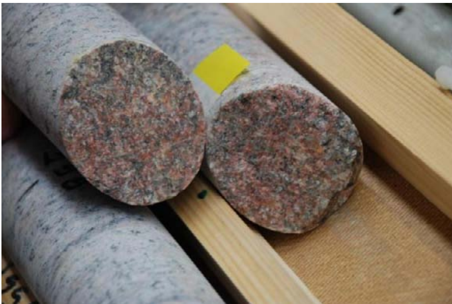
Figure 5-8. Photo of core KFM06A (fracture ID 945642D98A3485D4). This fracture is a typical Group 5 fracture, with no indications of mineral coating (i.e. a non-mineralised fracture by definition). This is a PFL-f fracture which was sampled for further mineralogical analyses. No signs of mineral coating were detected using SEM-EDS. Figure 5-9 shows the BIPS image of the same fracture. The diameter of the drill cores is 50 mm.
