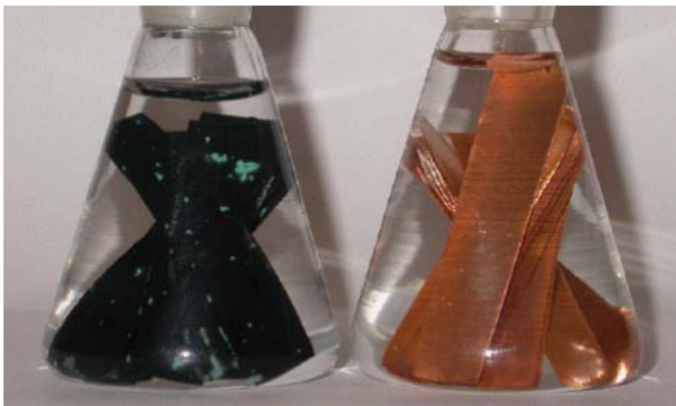
Figure 2-7. Appearance of copper strips after exposure to distilled water for 15 years at room temperature in Pd-sealed (left-hand side) or Pt-sealed (right-hand side) conical flasks (Figure 1 in Hultquist et al. (2008)).
