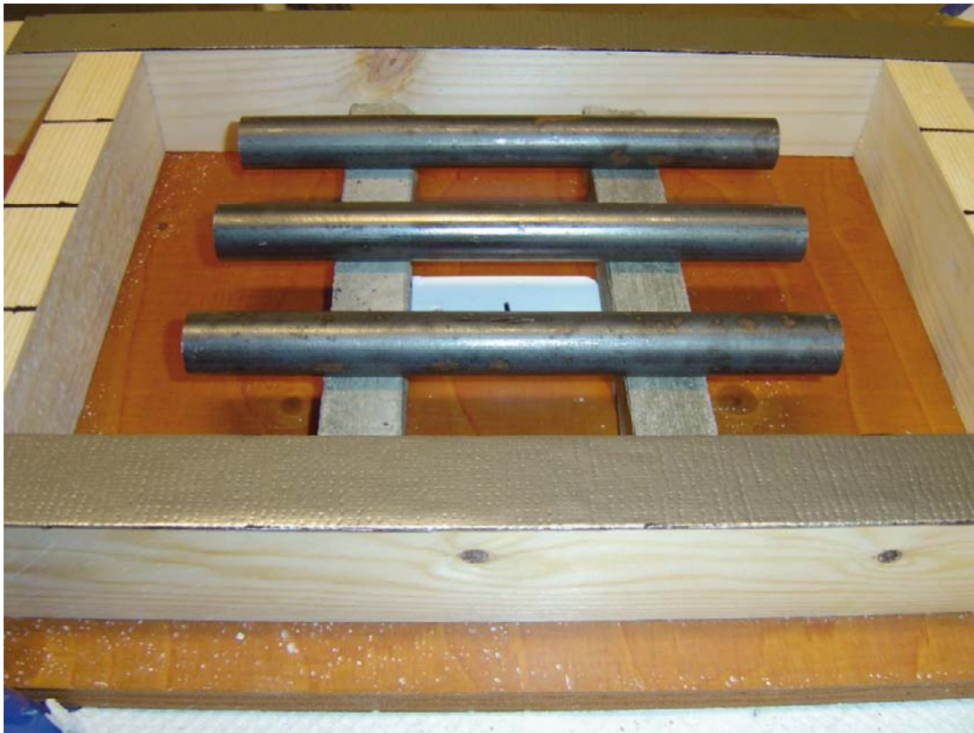
Figure 5-7. Mould and steel bars on supports before casting.
