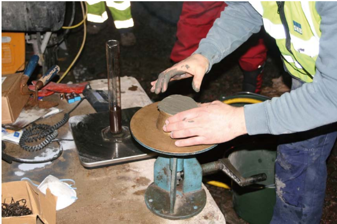
Figure 3-7. Flow test for checking consistency.
