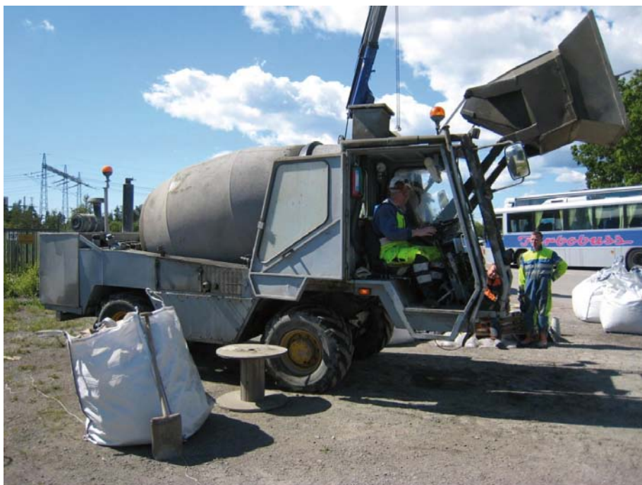
Figure 4-9. Mobile concrete mixing station, Terex Mariner 55. Also used for transporting the shotcrete to the shotcreting robot.
