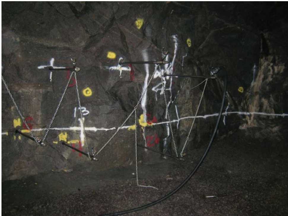
Figure 3-6. Secured packers used for hydraulic characterisation.
