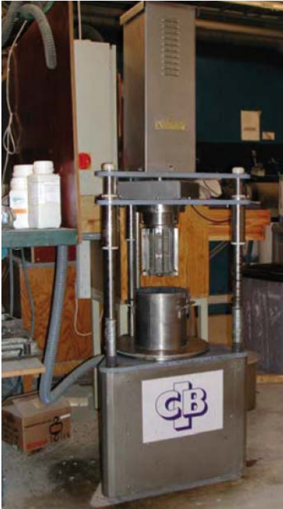
Figure 4-1. ConTec Viscometer 4 SCC. Courtesy of Björn Lagerblad and Mikael Westerholm, CBI.
