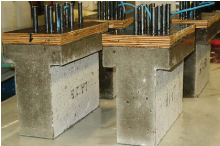
Figure 5-2. T-shaped specimens with steel bars for measuring chloride threshold. A total of eight bars were installed in each specimen. The concrete cover for each two bars was 10, 15, 20 and 25 mm respectively.
