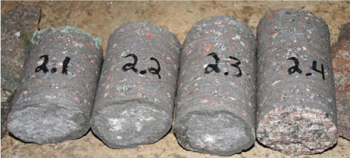
Figure 4-11. Drill cores from adhesion tests.
