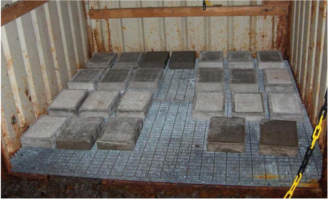
Figure 5-8. Container in Äspö HRL with samples corrosion tests.
