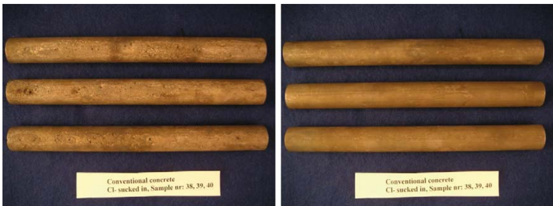
Figure 5-9. Example of photos of exposed steel bars, photographed from two sides.
