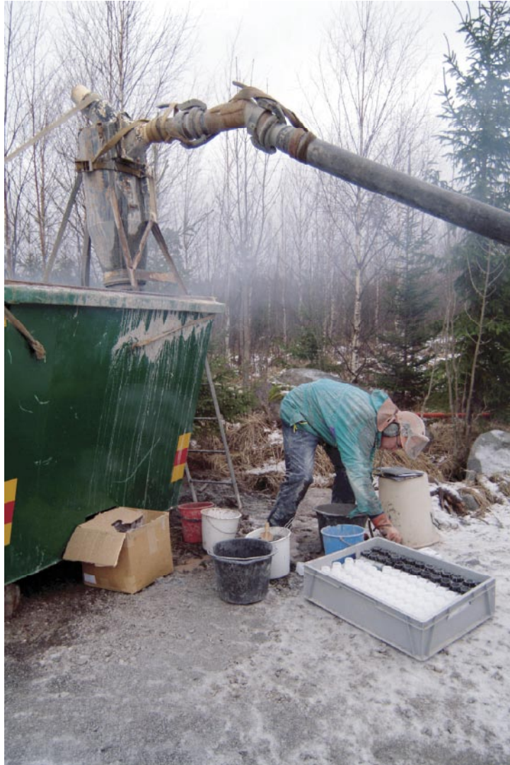
Figure 4-3. Sampling of one sample per 3 m drilling length of drill cuttings from the bedrock.
