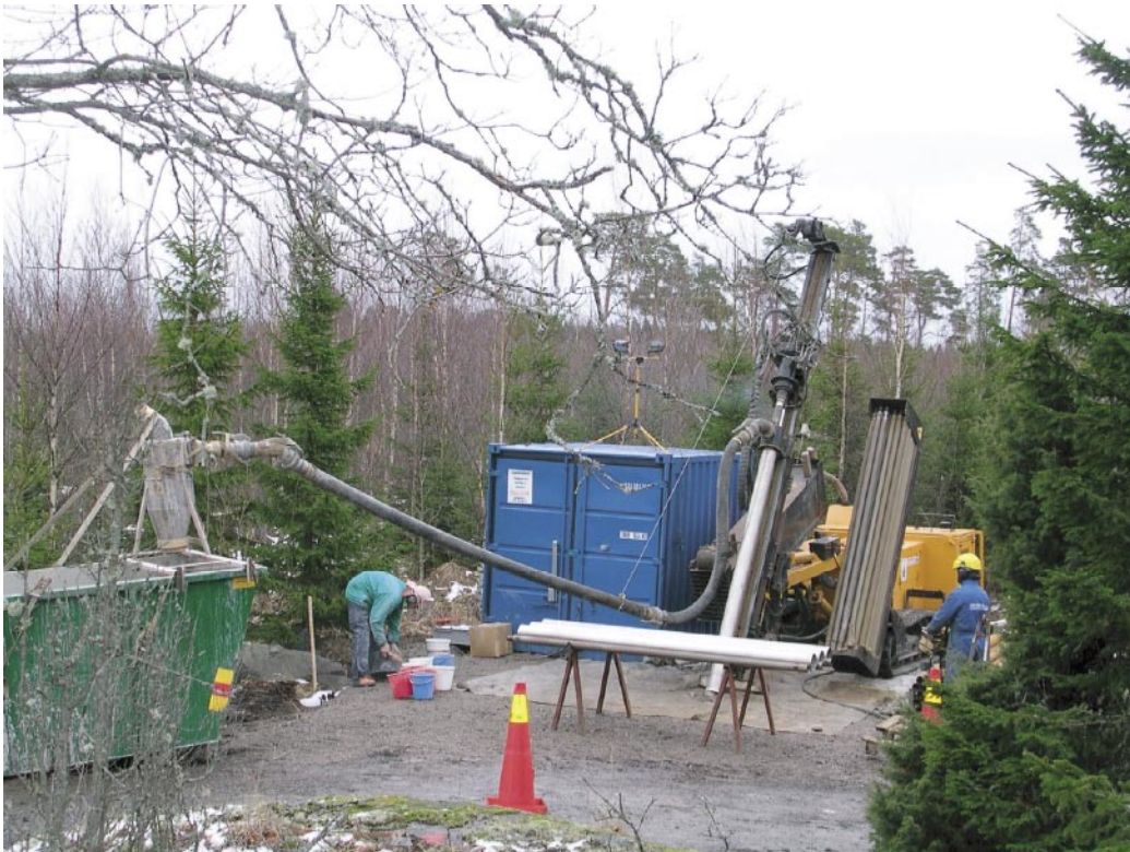
Figure 3-1. The Nemek 407 percussion drilling machine employed for drilling boreholes HFM11–12 and HFM17–18.
