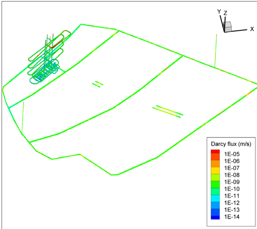
Figure 4-17. Magnitude of Darcy flux between open tunnels and the surroundings during glacial conditions.
