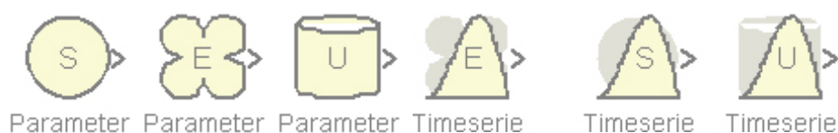
Figure 3-10. Illustration of the set of input variable blocks in Pandora. From left to right we have the Site-specific, Element-specific and Universal constant parameter blocks, and then we have the Element-specific, Site-specific and Universal constant time-series blocks.
