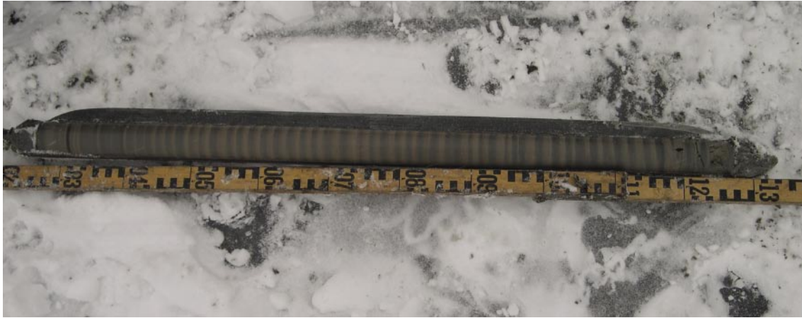
Figure 5-5. In Lake # 5, coring site PFM004205, the sedimentary sequence between 1.27–2.27 m depth consists of varved glacial clay. Bottom is to the right in the picture. The calcite content varied between 14 and 38% and the clay content varies between 74 and 43%. XRD analyses were performed on two samples from the coring site; one from a level above the photography (1.1 m) and one sample represents the proximal varves (1.37–1.5m). In both samples, Illite was the most common clay mineral.
