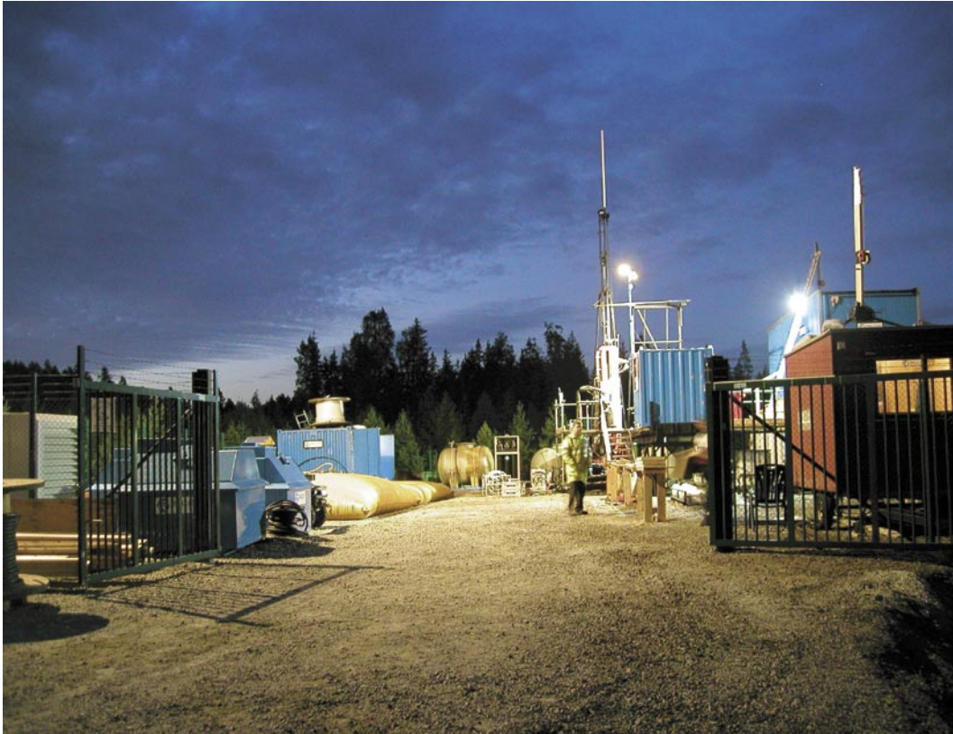
Figure 1-5. Drilling site DS1 with the complete core drilling outfit mobilized.
