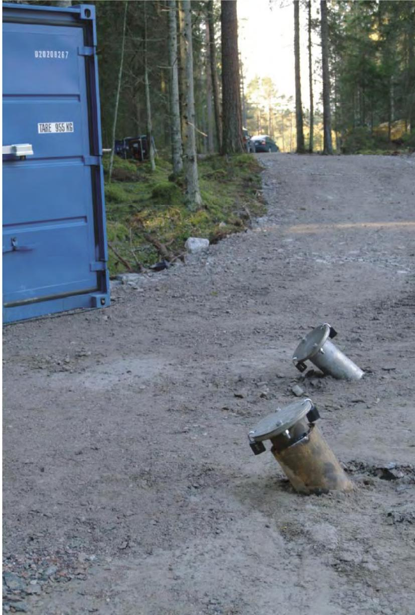
*Figure 4-4. After drilling and sampling, each borehole was secured by a stainless steel lockable cap, mounted on top of the casing flange.*
