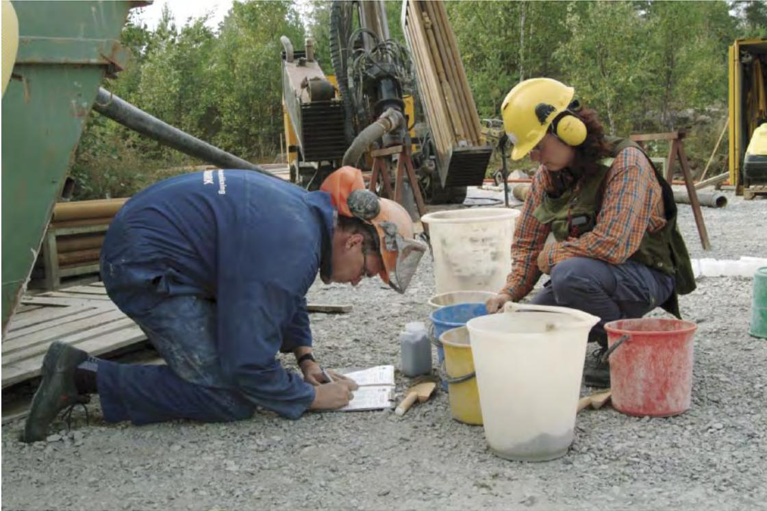
*Figure 4-2. Sampling of one sample per 3 m drilling length of drill cuttings from the bedrock.*
