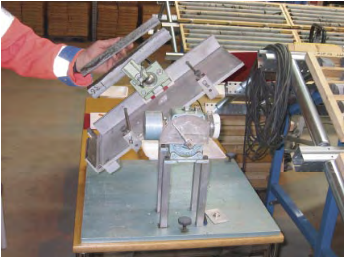
Figure 2-1. Sample for tilt testing in the tilt apparatus.
