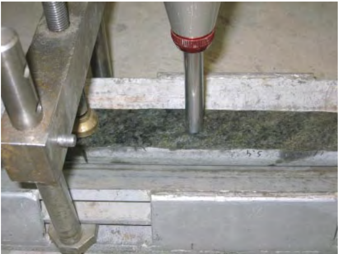
Figure 2-3. Clamp for the Schmidt hammer tests.
