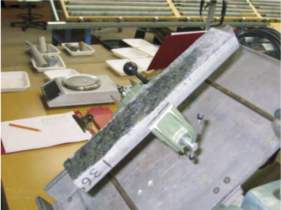
Figure 2-2. NGI's tilt test apparatus.
