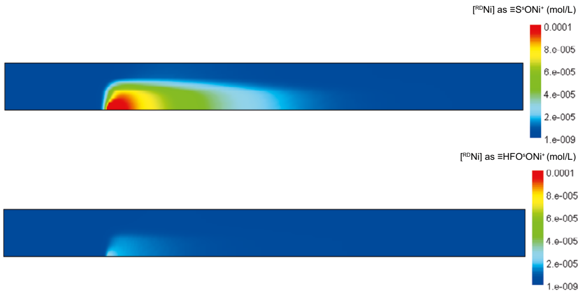
Figure 6-17. Concentration of ^{RD}Ni^{2+} retained in illite and ferrihydrite at the end of the simulation period (2,700 years after repository release).
