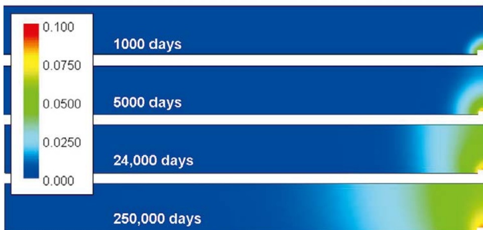
Figure 7-3. Migration of the conservative tracer in the clay domain at 100, 5,000, 24,000 and 250,000 days of simulation of deep groundwater input. Scale bar is concentration in mol/L.
