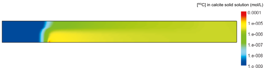
Figure 6-8. Concentration of ^{RD}C retained in calcite solid solution at the end of the simulation period (2,700 years after repository release).
