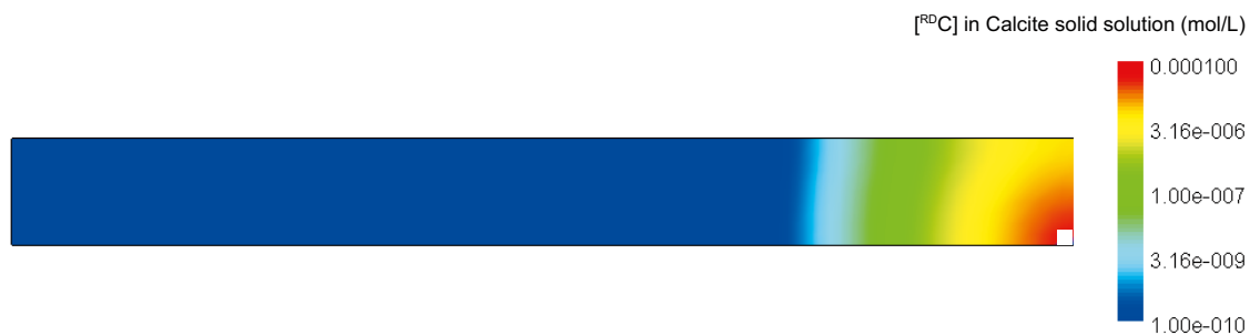
Figure 7-6. Concentration of ^{RD}\text{C} retained in the \text{Ca}^{(14}\text{C},\text{C})\text{O}_3 solid solution at the end of the simulation period (2,700 years after repository release).
