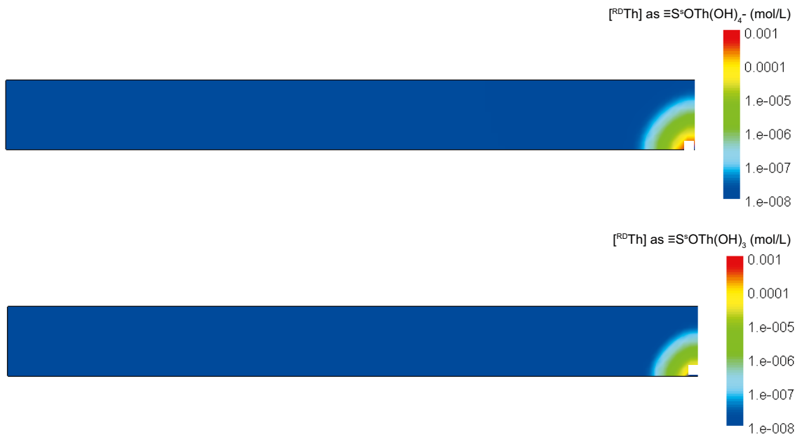
Figure 7-12. Concentration of two ^{\text{RD}}\text{Th} complexes retained in illite at the end of the simulation period (2,700 years after repository release).
