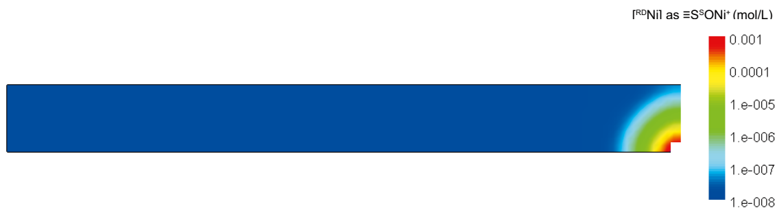
Figure 7-16. Concentration of ^{RD}\text{Ni} retained in illite at the end of the simulation period (2,700 years after repository release).
