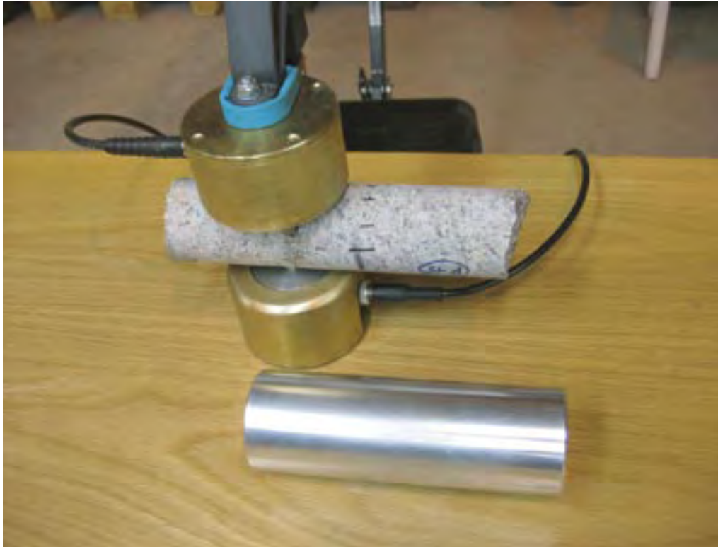
Figure 3-2. Detail of NGI's apparatus for measuring acoustic P-wave travel time transverse borehole core. The aluminium cylinder for calibration of the device is in front.
