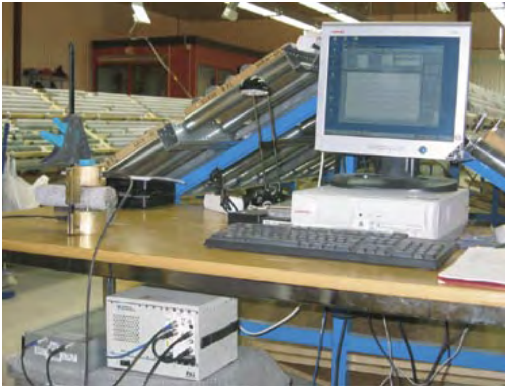
Figure 3-1. NGI's equipment set up for measuring acoustic P-wave travel time transverse borehole core.
