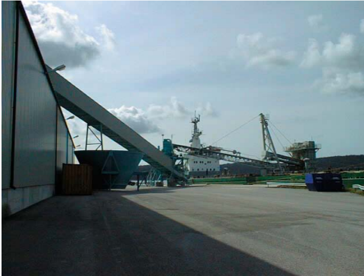
Figure 5-4. A self-discharging and loading vessel at Norske Skog's receiving facility in Halden, Norway.
