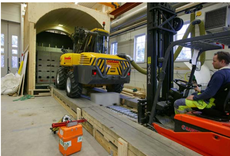
Figure 5-17. A stacking test being performed on a bentonite bed with a water inflow.
