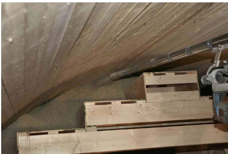
Figure 5-18. Pellet installation test with the reference equipment, at the Bentonite Laboratory at Äspö.
