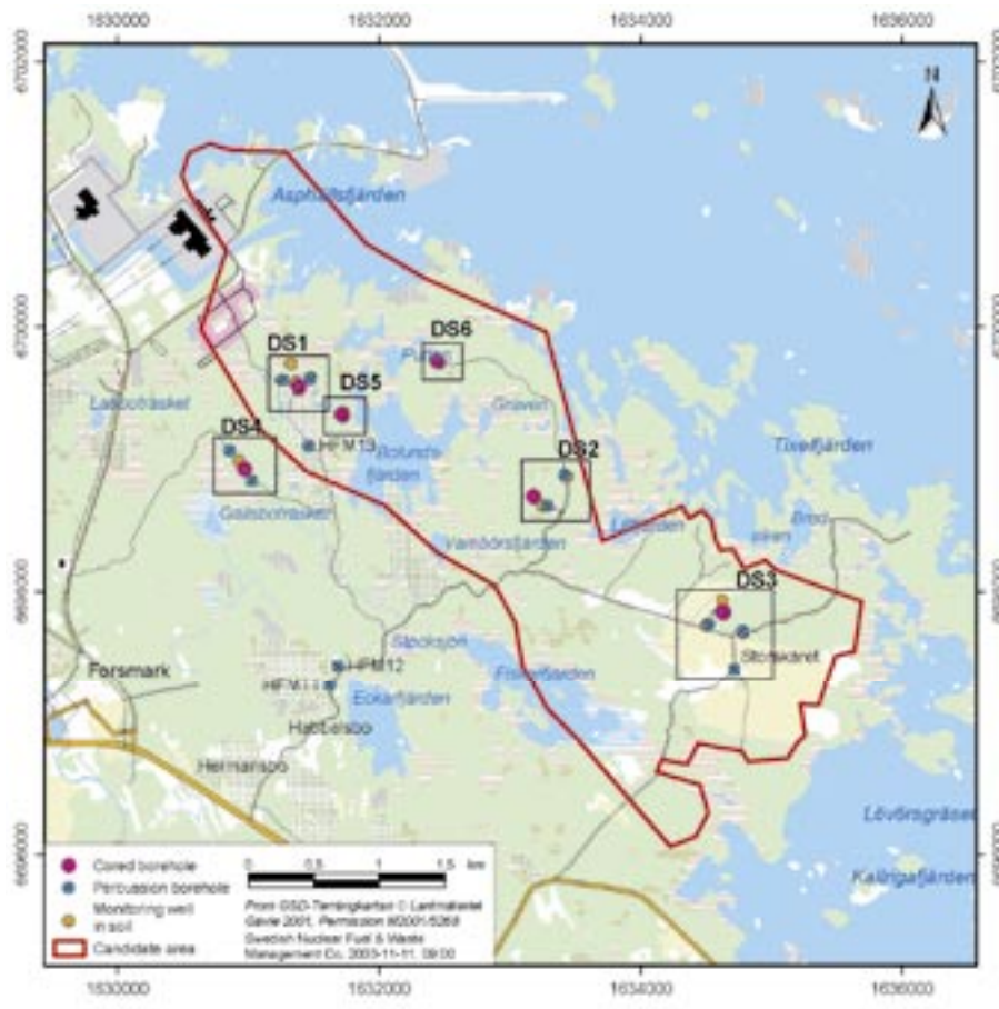
Figure 5-2. Overview of the Forsmark candidate area and location of boreholes (situation autumn 2003).
