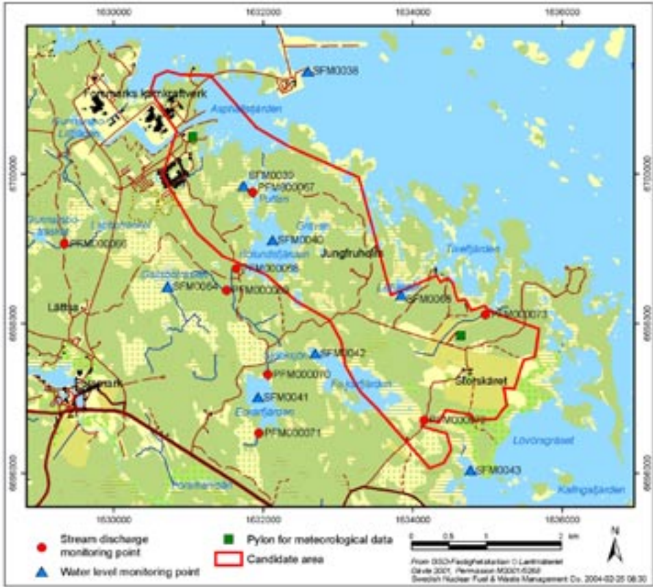
Figure 5-6. Measuring stations for surface water discharge, water level and meteorological parameters of the Forsmark site investigation.
