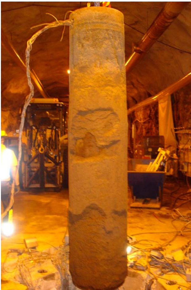
Figure 4-15. Lifting of Heater 2.
