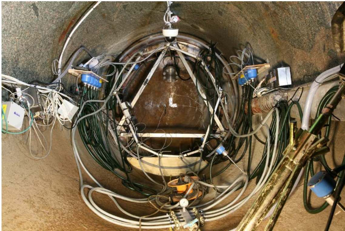
Figure 4-18. Fully instrumented compartment plug in DA1622A01.
