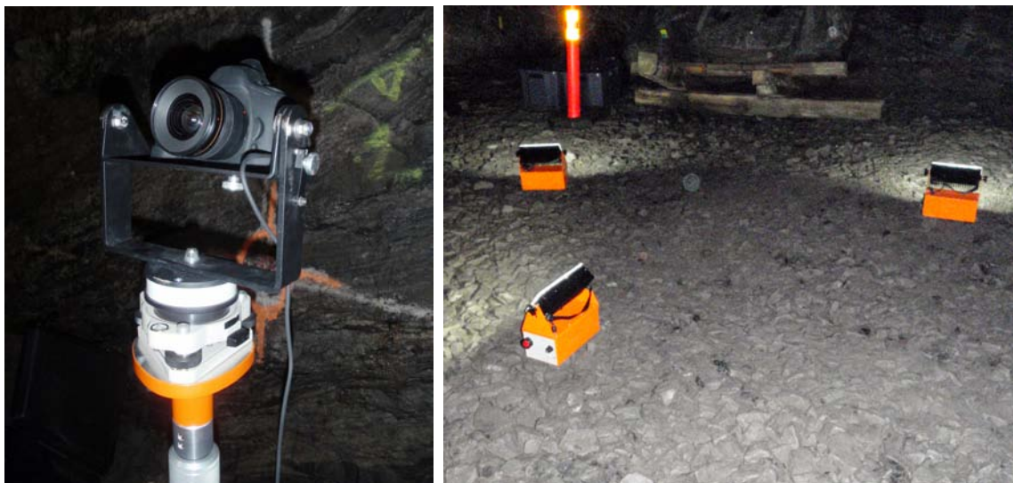
Figure 2-2. Adam Technology’s field equipment; digital camera on a tripod (left) and portable illumination (right).
