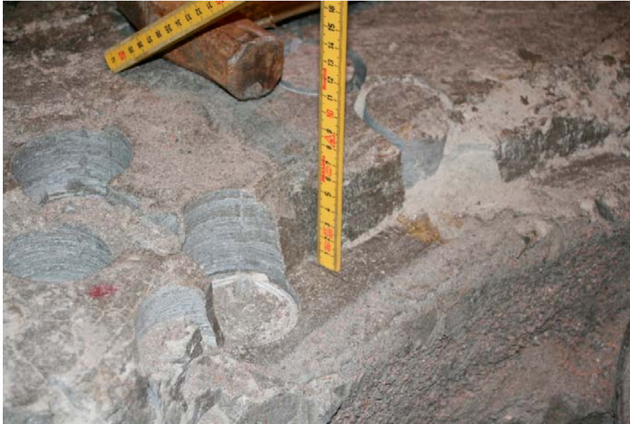
Figure 4-16. Traces of shear deformation in Ring 12.
