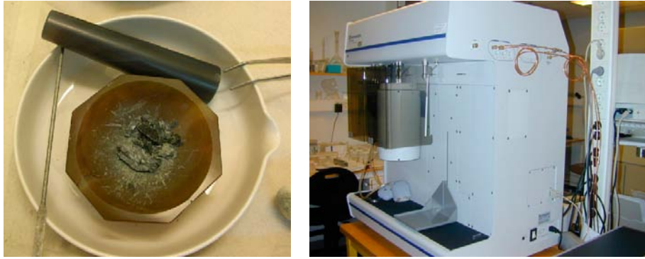
Figure 3-9. Powder preparation from a chlorite specimen in an agate mortar (left). Instrument for making surface area determinations (right).
