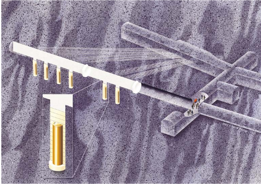
Figure 4-1. Schematic view of the layout of the Prototype Repository (not to scale).
