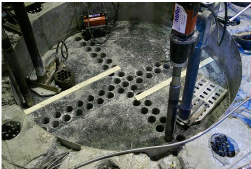
Figure 4-14. Core sampling in Cylinder 4.
