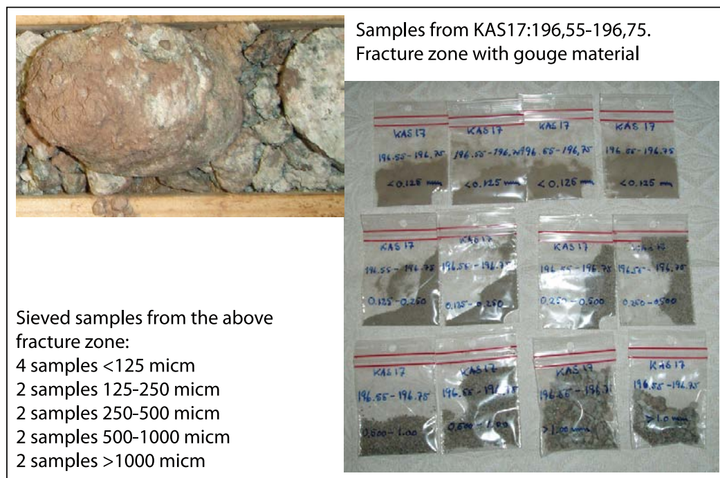
Figure 3-7. Photo of samples from a fracture zone at a depth of 196.55–196.75 m in KAS 17.
