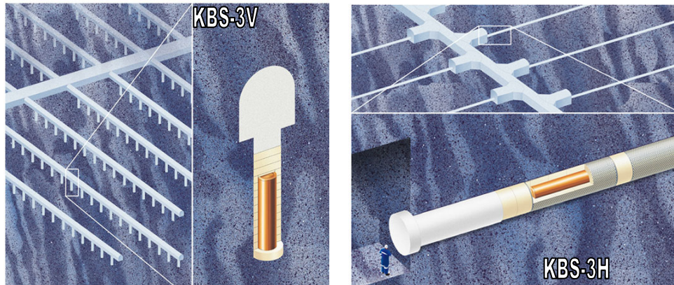
Figure 2-5. Schematic illustrations of variants of the KBS-3 method.
