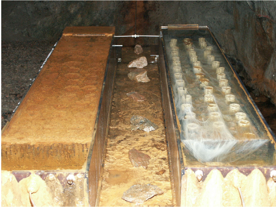
Figure 4-12. The artificial channels at 2200-m MICROBE site are fed by water from a common borehole, but they are inhabited by either iron oxidising microbes (left) or sulphur oxidising microbes (right). The balance between iron and sulphur microbes is very delicate. A small difference in the inlet profile of ground water results in a huge difference in the structure of the respective population.
