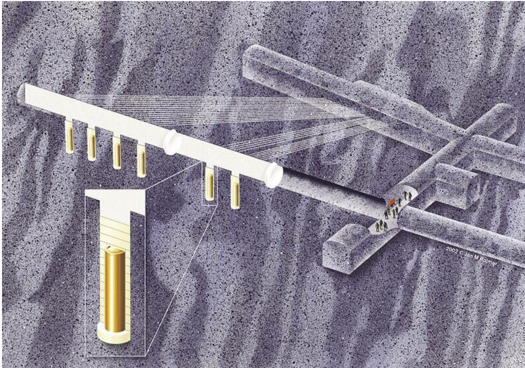
Figure 2-2. Schematic view of the layout of the Prototype Repository (not to scale).
