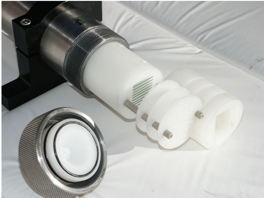
Figure 4-11. One of the twelve flow cells that are installed at the MICROBE 450-m site. Ten pieces of surfaces can be installed. They can be made of granite, glass metal or combinations, depending on the aim of the experiment. Three flow diffusers before and after the surface pile distributes the flow evenly over the test surfaces.
