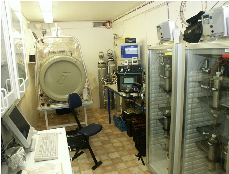
Figure 4-10. An overview of the laboratory environment at the MICROBE 450-m site. The laboratory is equipped with three circulation systems (right), an anaerobic box (forward), an in situ gas extractor and a Kappa 5 gas chromatograph (right of the anaerobic box).
