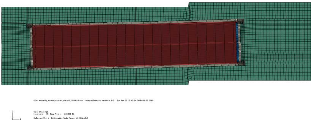
Figure A8-2. Deformed plot – 10 cm shearing magnitude.
