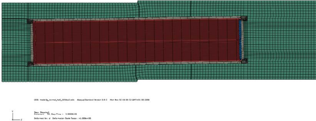
Figure A2-1. Deformed plot – 5 cm shearing magnitude.
