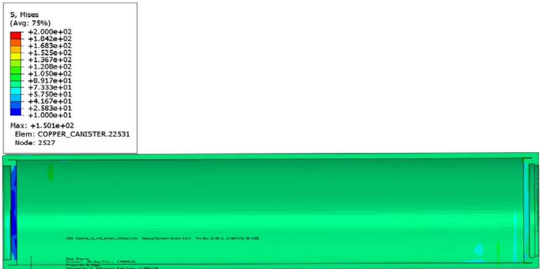
Figure A4-3. Mises stress for copper shell – 5 cm shearing magnitude.
