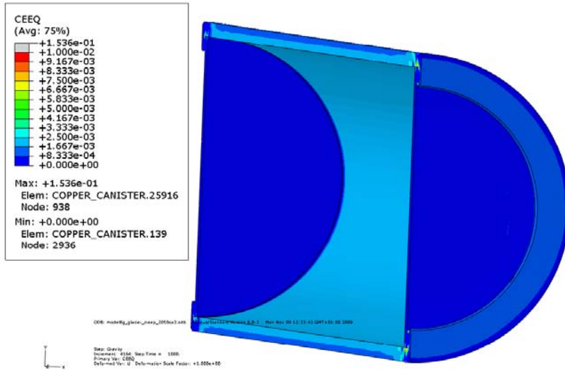
Figure 9-12. Equivalent creep strain (CEEQ) after applying the glacial load (1,000 seconds).
