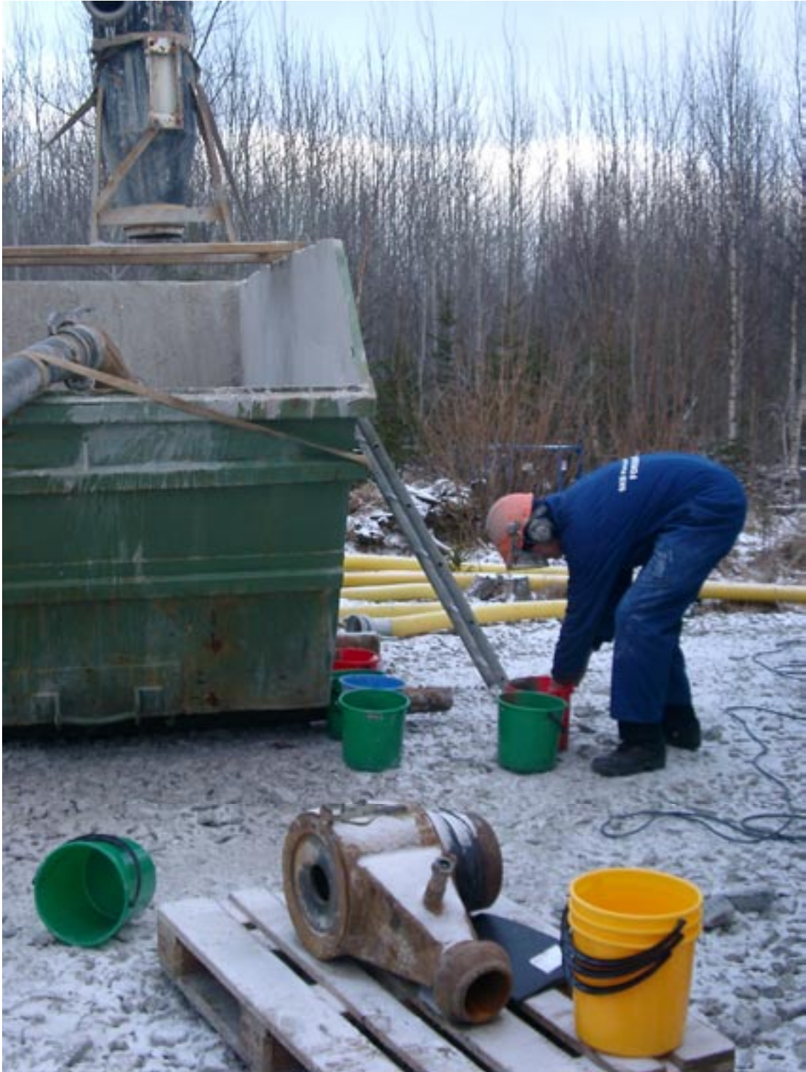
Figure 4-3. Sampling of one sample per 3 metre drill length of drill cuttings from the bedrock. Photo Alf Sevastik.
