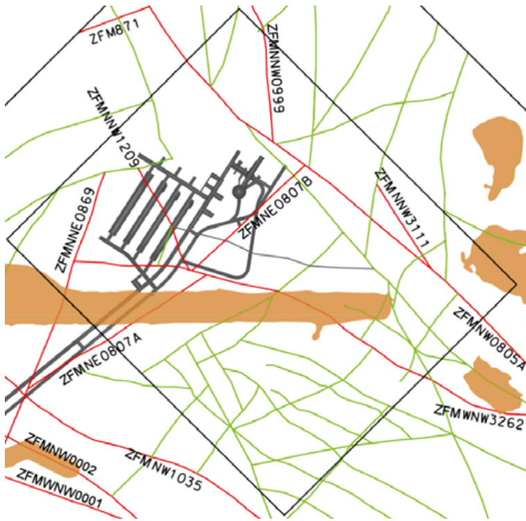
Figure 2-4. Local model area (version 0.1) showing the intersection at the current ground surface of deformation zone traces. Degree of confidence: high=red, medium=green, low=grey /Curtis et al. 2009/. Light brown=Land, White=Sea.
