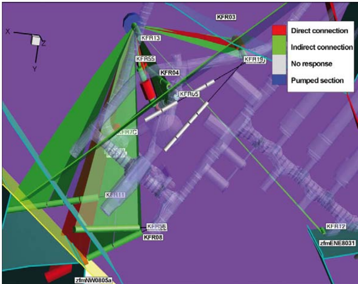
Figure C-6. Interference test in KFR13 (54–76.6 m) covering 72% of the hydraulic envelope of ZFM871 (top view). Long distance observations KFR12 (250 m) and KFR08 (215 m).
