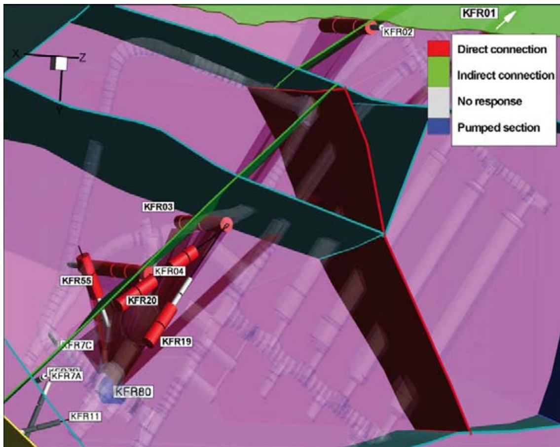
Figure C-8. “Unintentional interference test” in KFR80 (1.5–20 m) entirely inside ZFM871. Several direct responses in zfmne0870. Longest hydraulic paths to KFR02 (zfmne0870a; 300 m) and KFR01 (zfmwnw0001; 860 m).
