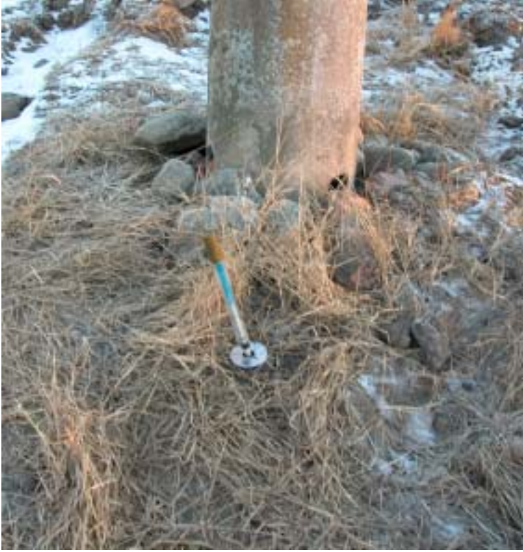
Figure 3-1. Measuring device for registration of frost depth in the ground.
