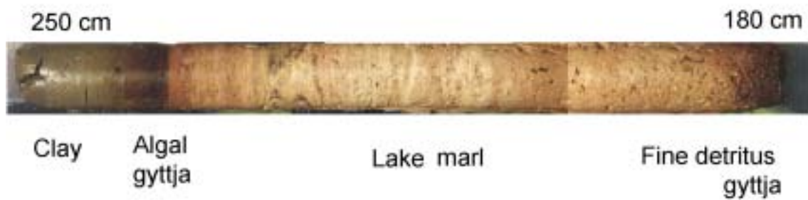
Figure 4-1. Photo compilation of the sediment sequence between 250 and 180 cm depth from Lake Barsjö. Approximately 1 meter of partly unconsolidated fine detritus gyttja has been accumulated on top of the lake marl. The water depth at the sampling site was 90 cm.
