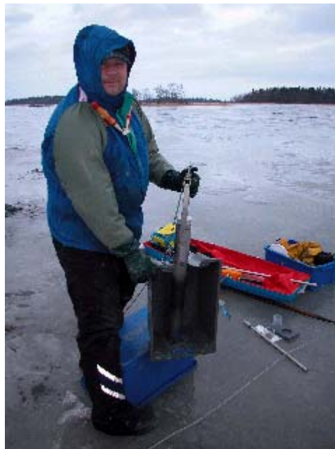
Figure 3-1. Compact modified stainless steel “Kajak samplers” with 70–100 cm long metal free polycarbonate tubes were used for collecting sediment cores through the sometimes thick ice cover of sea and lakes. Photo from Kallrigaffjärden, January 2003.
