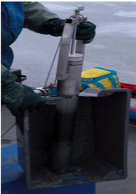
Figure 3-1. Compact modified stainless steel “Kajak samplers” with 70–100 cm long metal free polycarbonate tubes were used for collecting sediment cores through the sometimes thick ice cover of sea and lakes. Photo from Kallrigaffjärden, January 2003.
